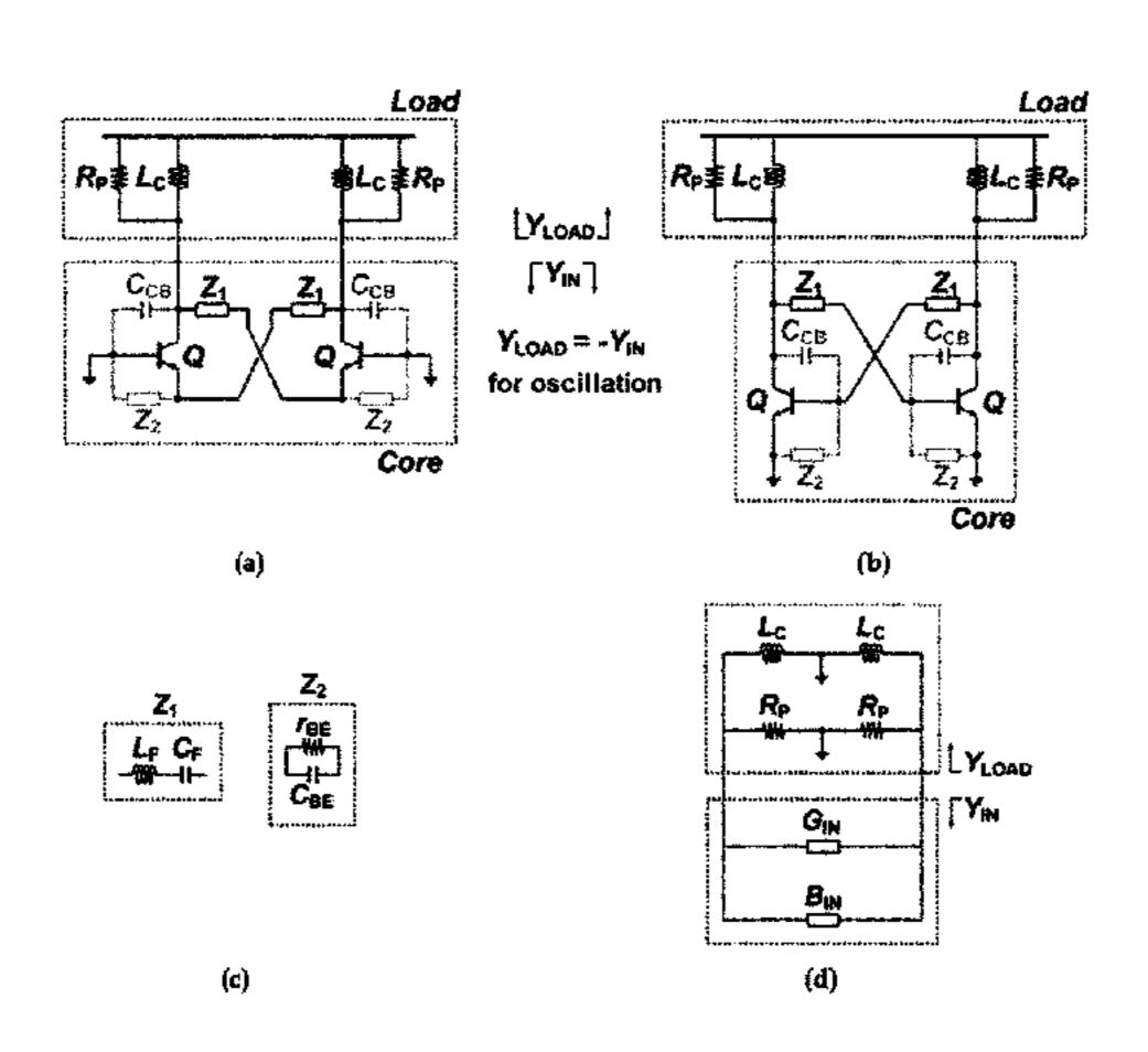
connected to a ground, and a second emitter connected to the second base, the oscillator having a common-base cross-coupled structure in which the first collector and the second emitter are cross-coupled and the second collector and the first emitter are cross-coupled.
