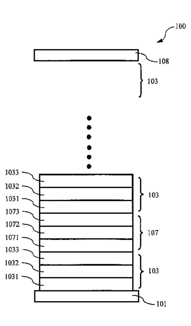
an inverted-type stacked organic light-emitting diode (the lower electrode is a cathode).
