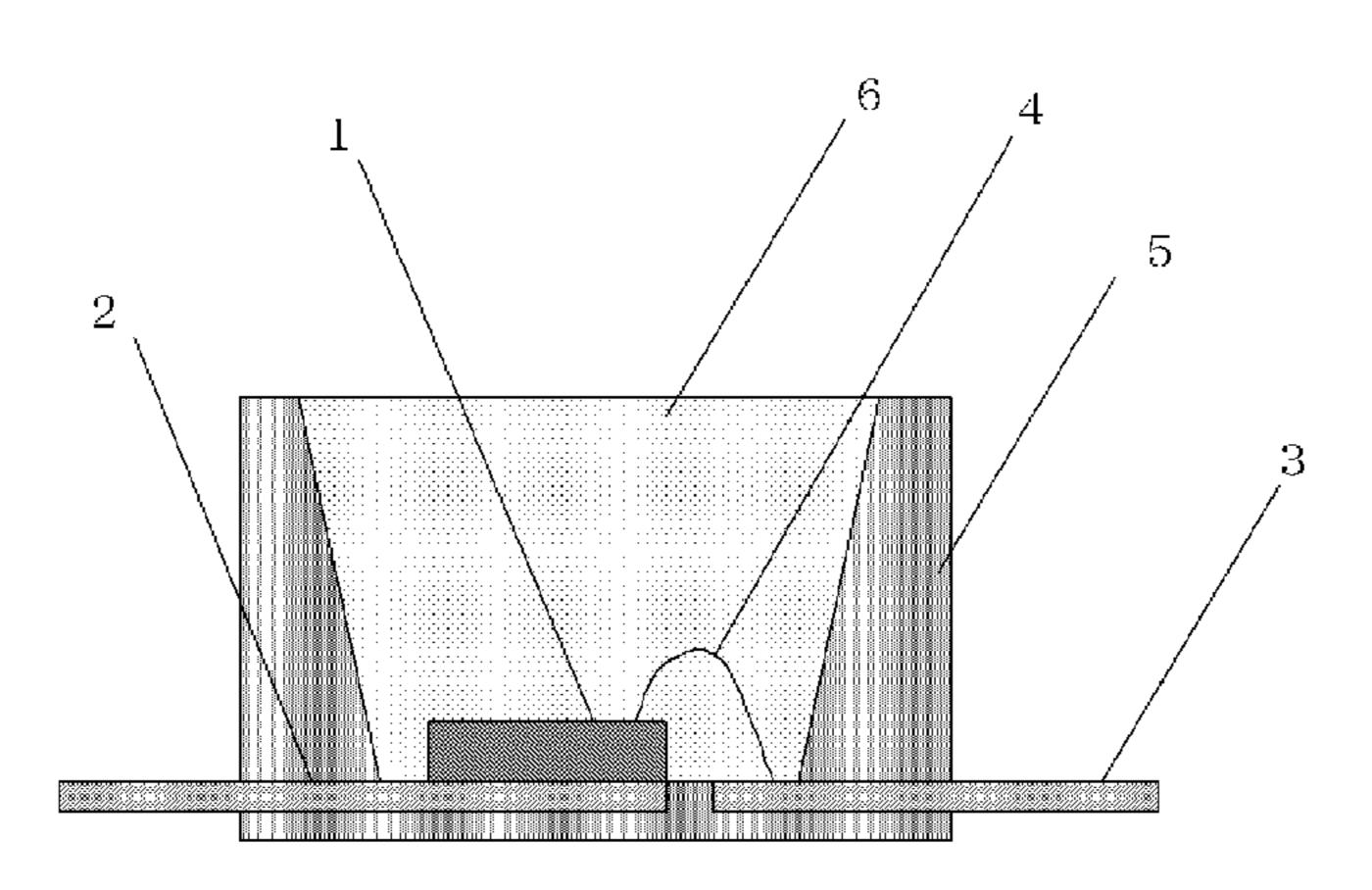
ductor element is sealed, covered, or adhered by the cured product of the composition so that the discoloration of silver electrodes or a silver-plated substrate due to a sulfur-containing gas in the air is inhibited.
