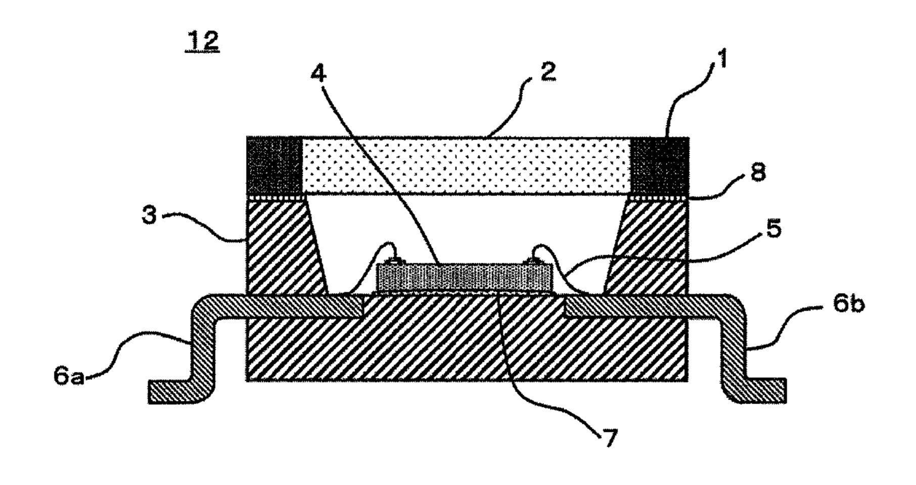
into individual pieces, fitting the glass piece into the opening of the phosphate-based glass (1) having light-shielding properties, the opening having been formed so as to have a size approximately equal to the cavity size, and melting and integrating the glasses member.
