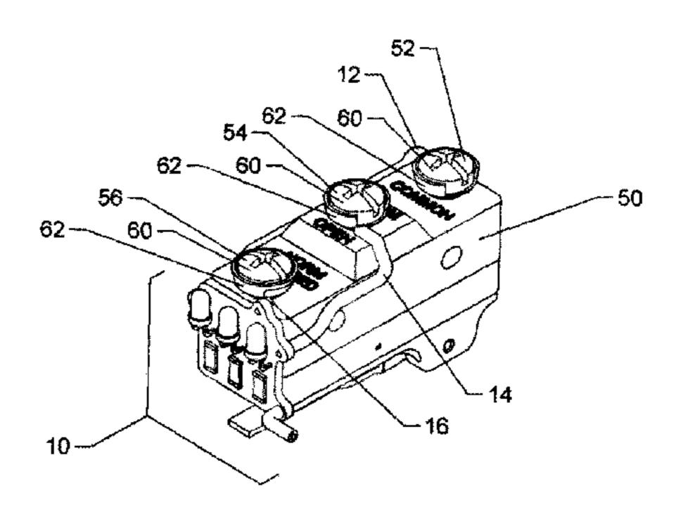
or both. These lights can respond to indicate the state and operation of the switch.
