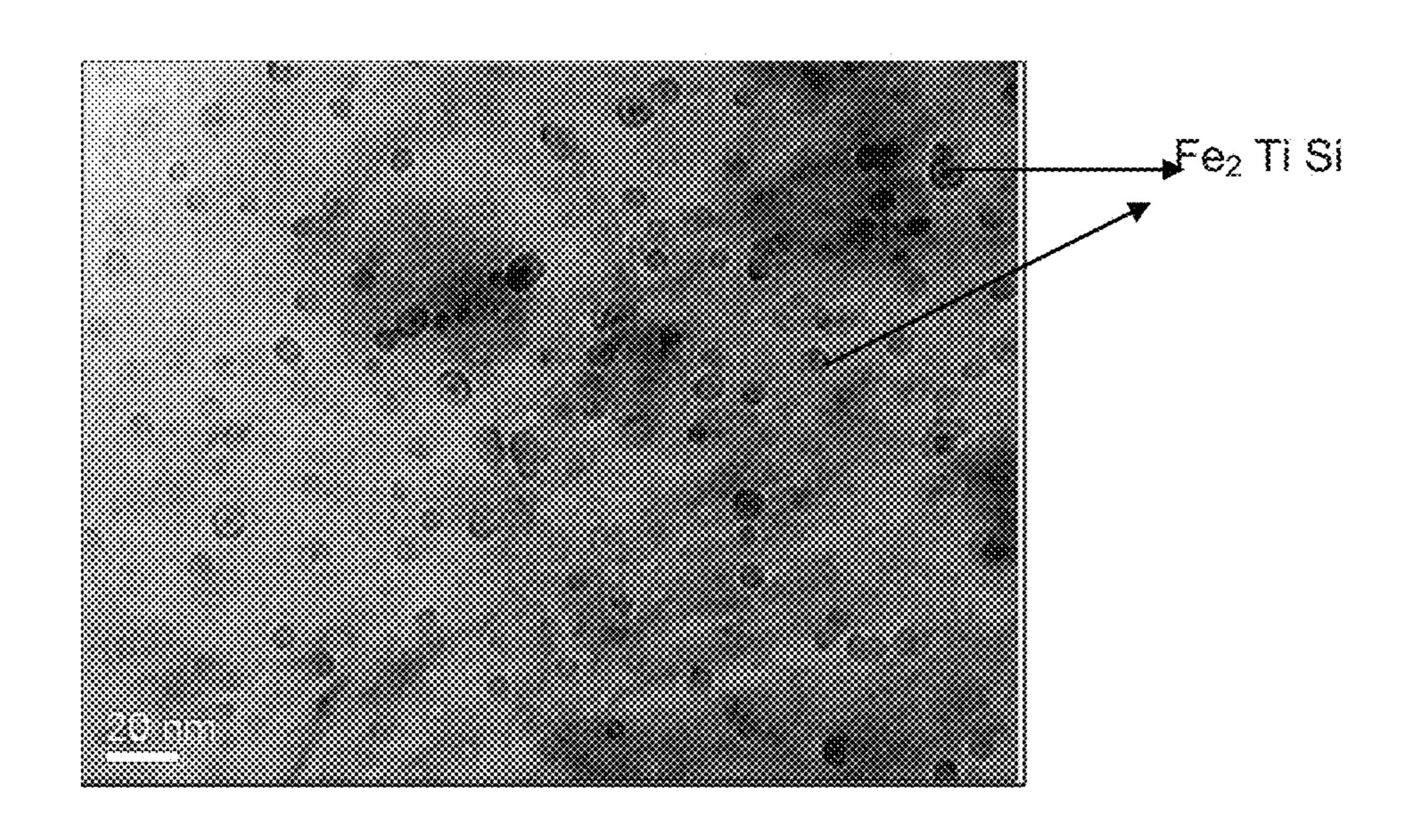
ROLLED STEEL THAT HARDENS BY MEANS OF PRECIPITATION AFTER HOT-FORMING AND/OR QUENCHING WITH A TOOL HAVING VERY HIGH STRENGTH AND DUCTILITY, AND METHOD FOR MANUFACTURING SAME
