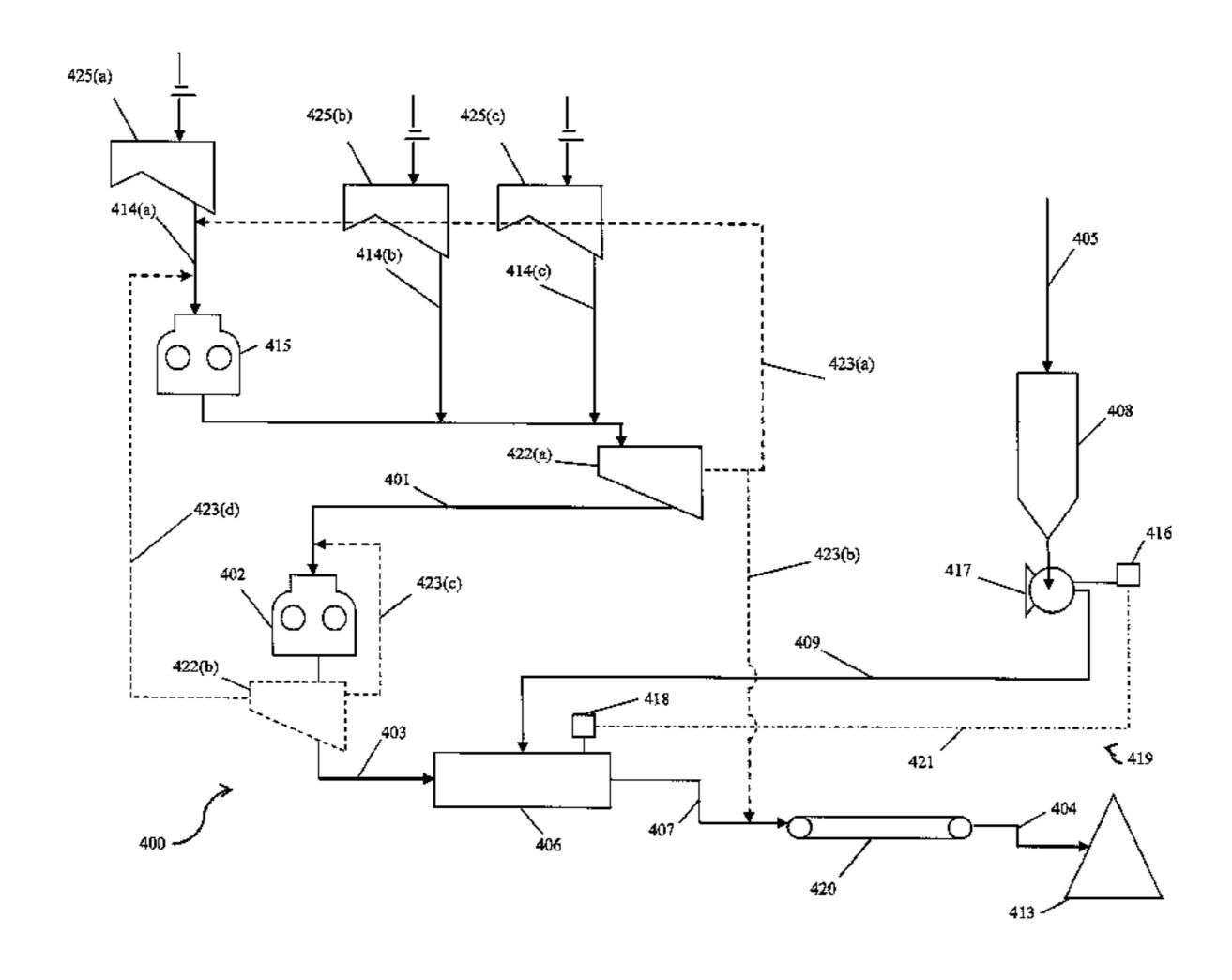
coarse tailings stream to form a combined tailings disposal stream. Dewatering apparatus may also be provided.
