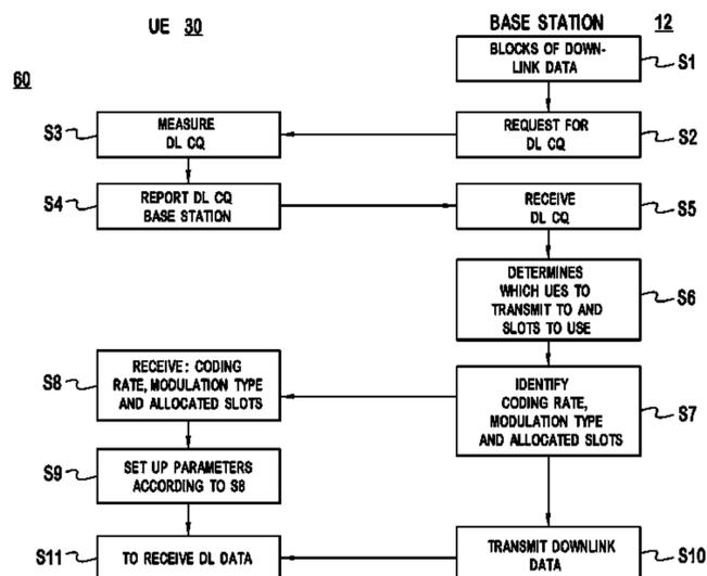
from those mobile terminals (UEs) with pending downlink transmissions. The UEs respond to the request by measuring and reporting DL channel quality to the base station, which then allocates resources such that the UEs will make best use of radio resources. The base station notifies the UEs of the physical channel allocation indicating the modulation/coding rate and allocated slots followed by transmission of blocks of downlink data which are transmitted to the UEs.
