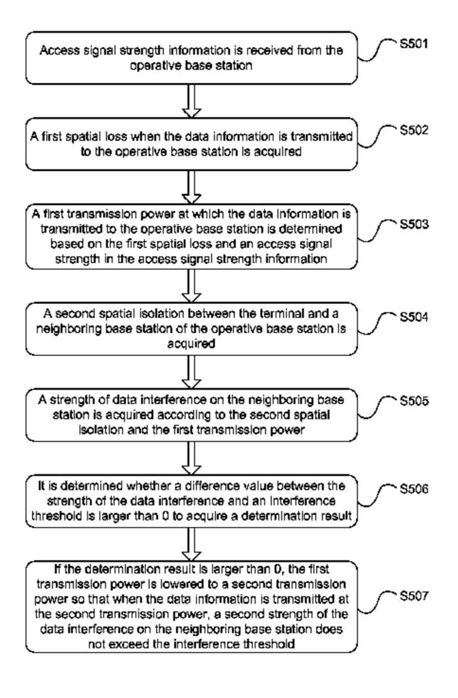
information is transmitted at the second transmission power, a second strength of the data interference on the terminal attributed to the neighboring base station does not exceed the interference threshold, thereby solving the technical problem in the prior art that there is too excessive interference on other terminals when a base station transmits data signals.
