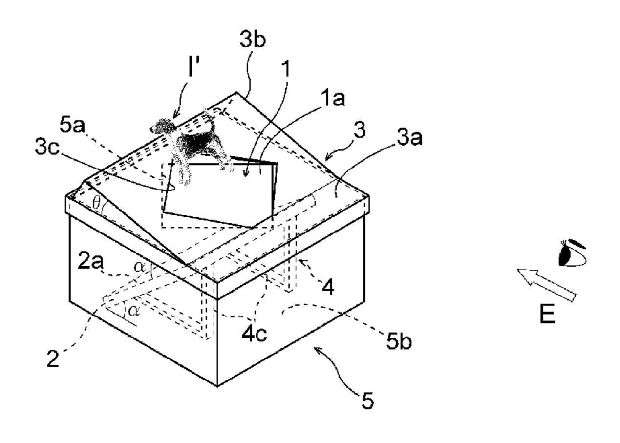
the back side with respect to the image-forming optical element, whereby the spatial image floats up through the opening of the guide plate. This allows anyone to view a three-dimensional spatial image rich in a sense of depth without experience and skill automatically in an appropriate direction from an appropriate position.
