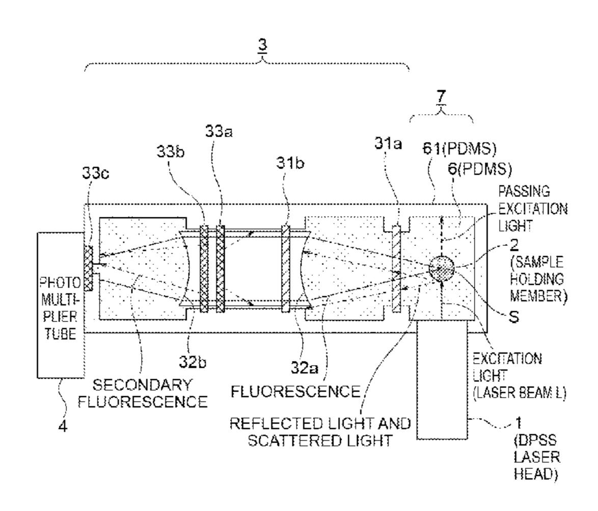
light generated from the resin, and so forth is contained substantially in a uniform manner in a resin region that surrounds the light path through which the excitation light and the light including the fluorescence pass.
