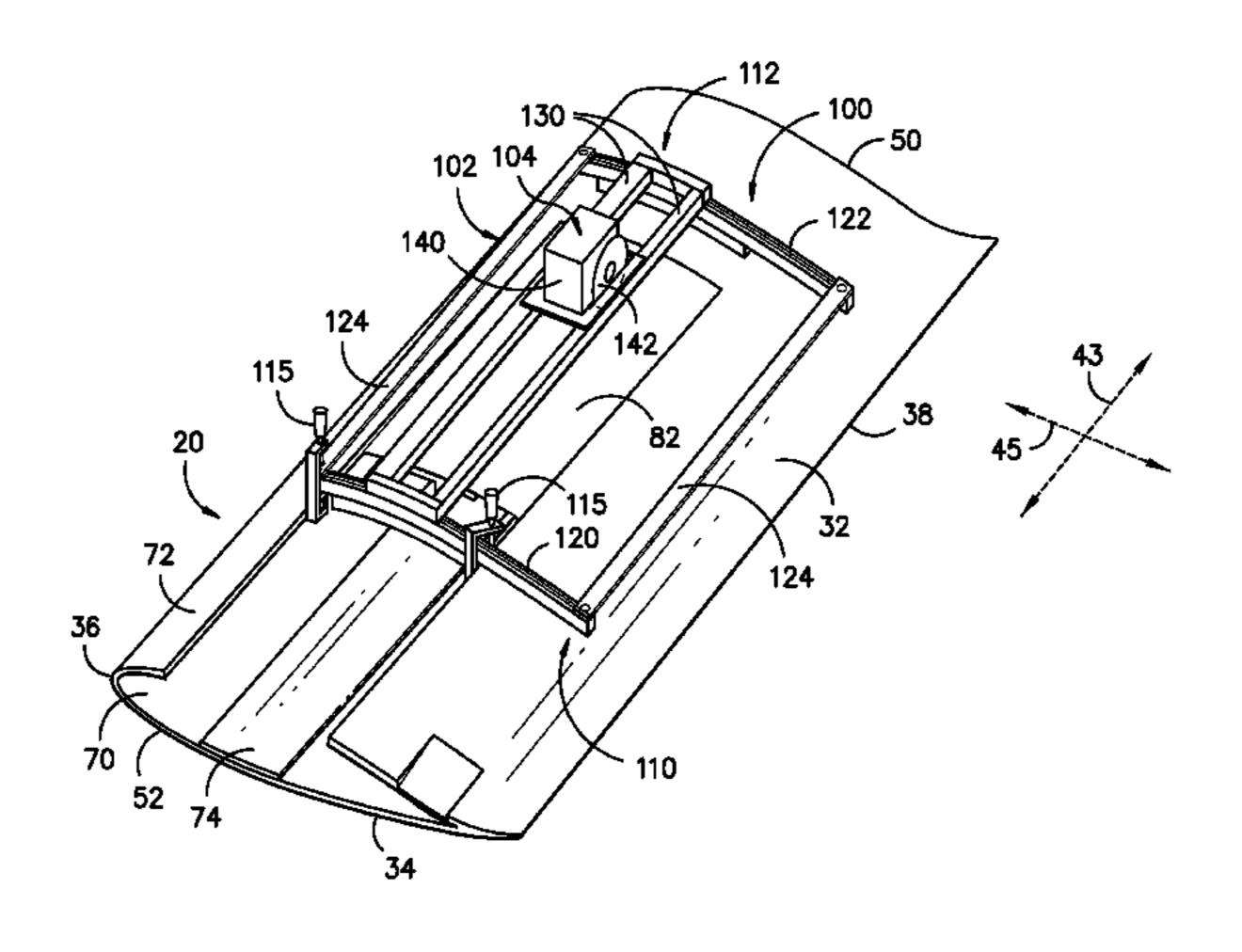
cutting device movable along the guide rail and operable to remove material from the one of the pressure side or the suction side.
