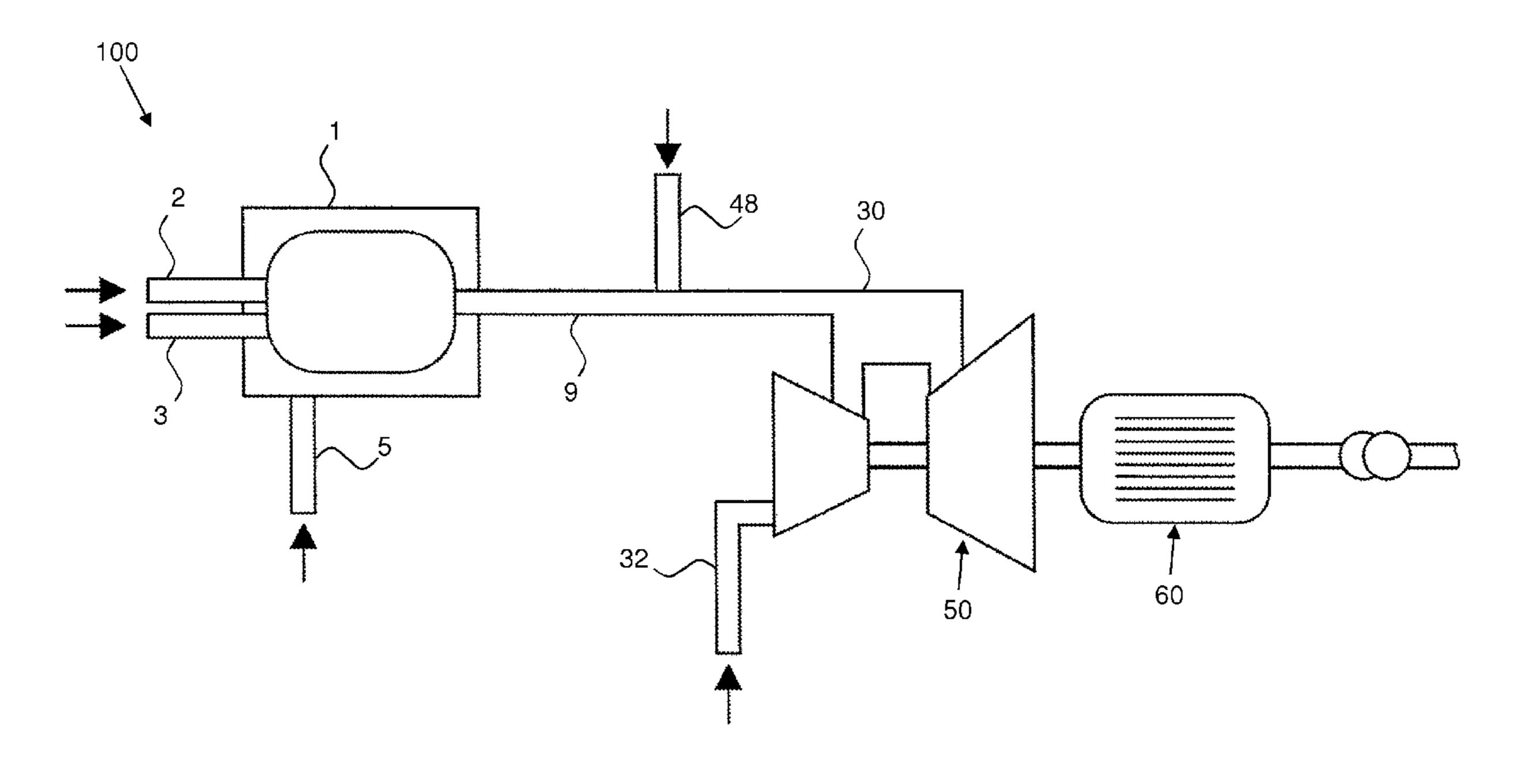
rotational movement to generate electrical power. The power plant is characterized according to the invention in that, in order to provide a heat supply, in addition to the reformer burning device, an electric heating unit is provided, through which electrical energy can be converted into heat energy.
