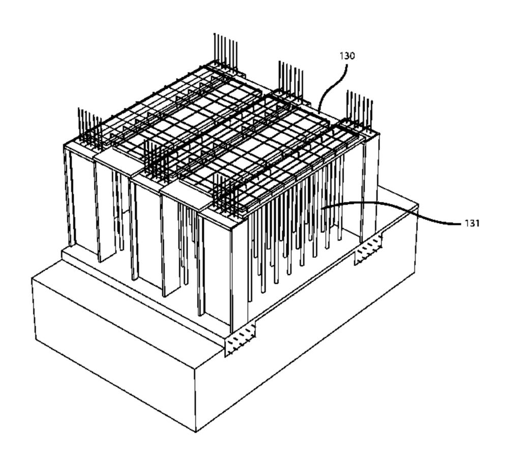
umns, beams, and floor slabs with minimal form work and construction site logistics. Also described herein are a method of assembly of said structures and a method of fabricating said assemblies.
