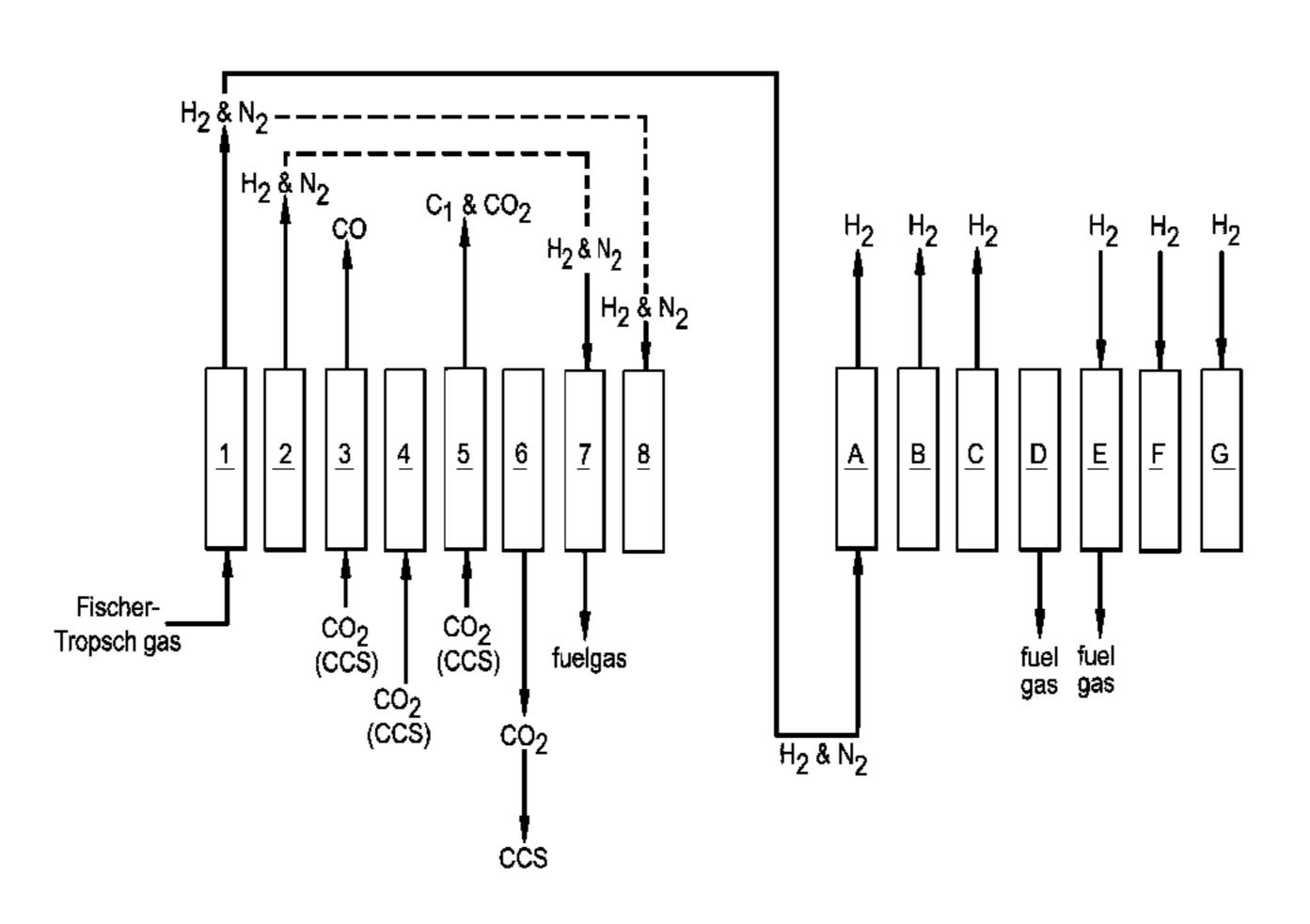
and carbon dioxide at a high pressure can be recovered from the Fischer-Tropsch gas. This can be fed to a gasifier or a reformer. In a preferred embodiment a gas comprising at least 80 vol % hydrogen is produced as well.
