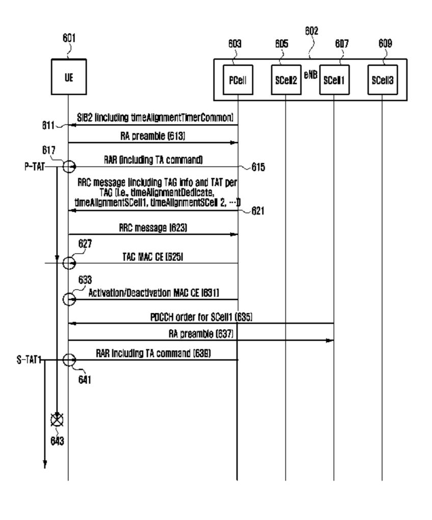
an index on a timing advance group (TAG), operating the timer for the TAG, the index has a value of 00 when the TAG includes a first cell. A terminal operates a timer by operating a first timer for a TAG including a first cell, operating a second timer upon receipt of a timing advance command for a second TAG that does not include the first cell, and, if the first timer has expired, deeming the second timer to also be expired.
