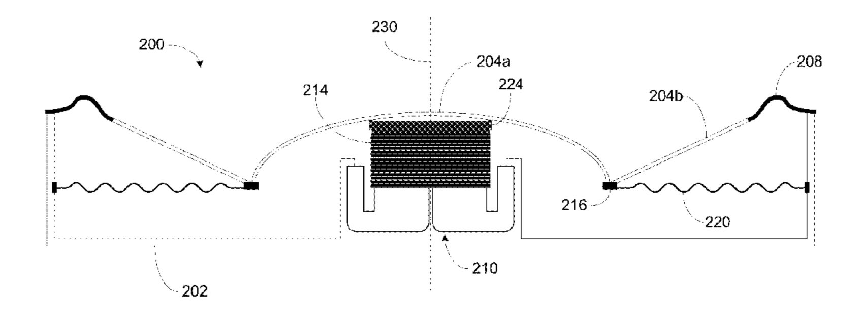
ential middle section of the diaphragm between the continuous central portion and outer portion of the diaphragm.
