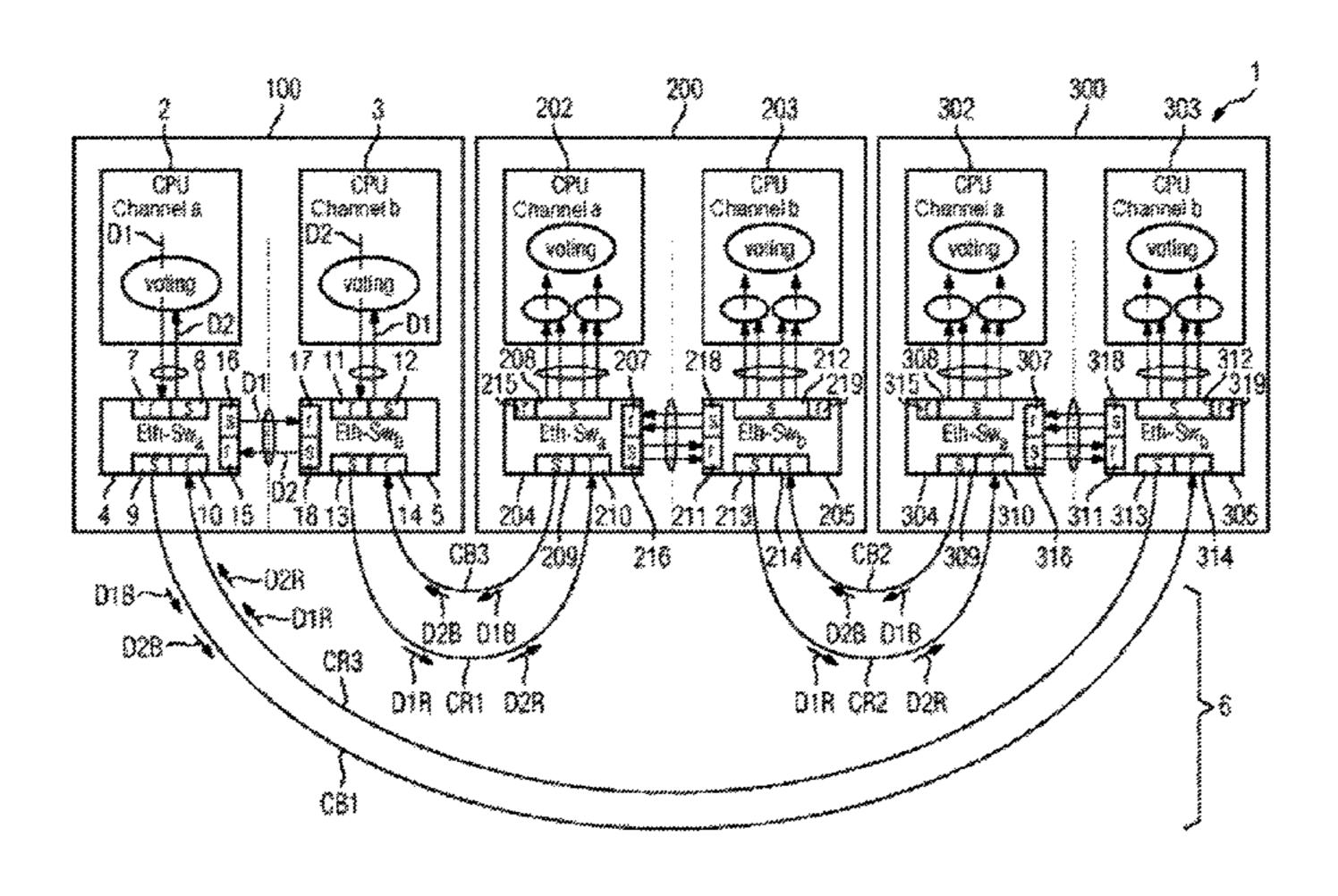
data exchange at the first and second internal transmitting and receiving port is prioritized over a data exchange at the transmitting and receiving port for transmitting and receiving data via the communication network.
