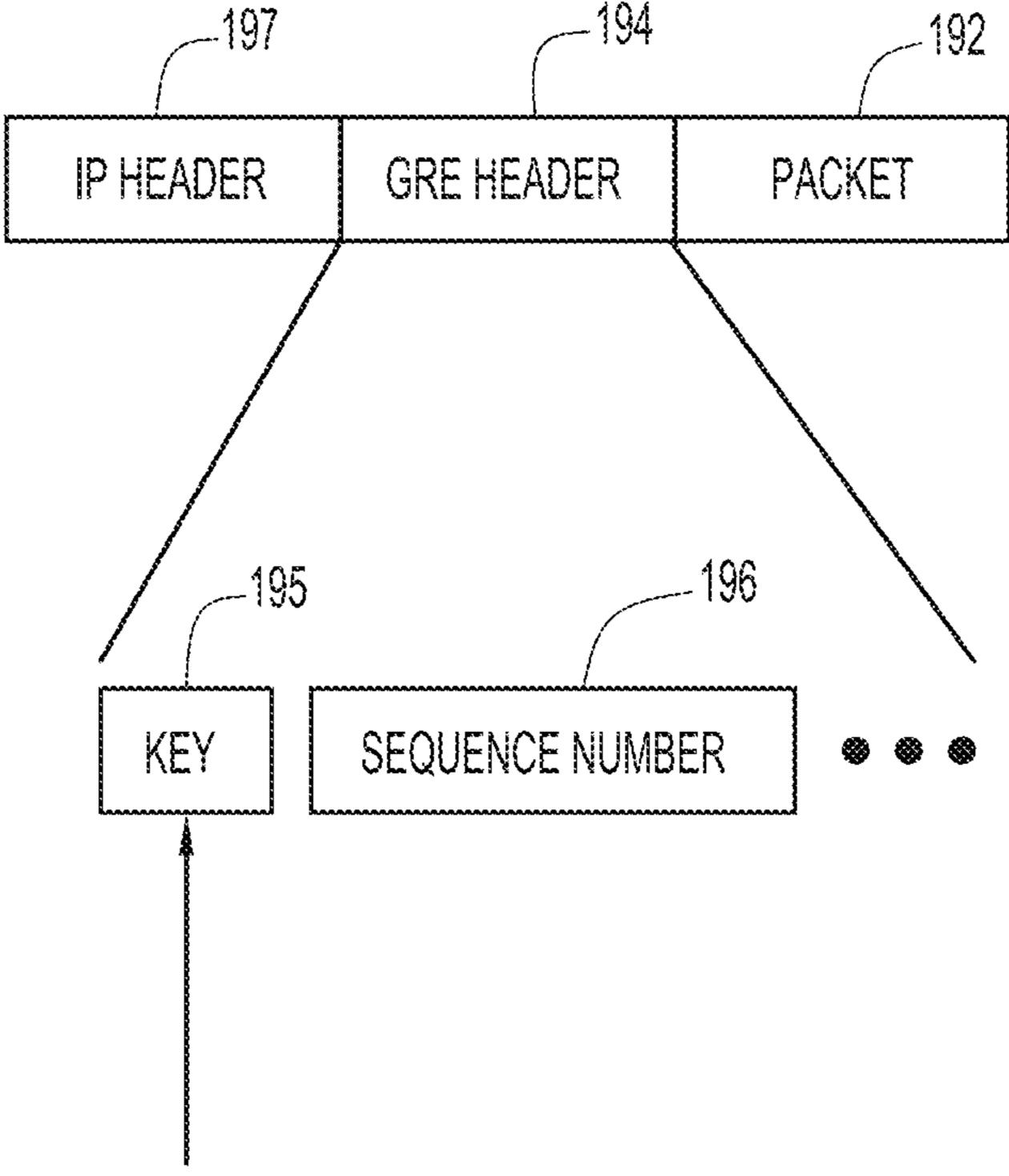
VALUE IN KEY FIELD FOR TRAFFIC SENT OVER GRE TUNNEL FORWARDING ROUTER: SETS VALUE FOR KEY ACCORDING TO ROUTING CONTROL TABLE RECEIVING ROUTER: DETERMINES ROUTING ACTION BASED ON KEY CONTAINED IN HEADER OF RECEIVED PACKET
