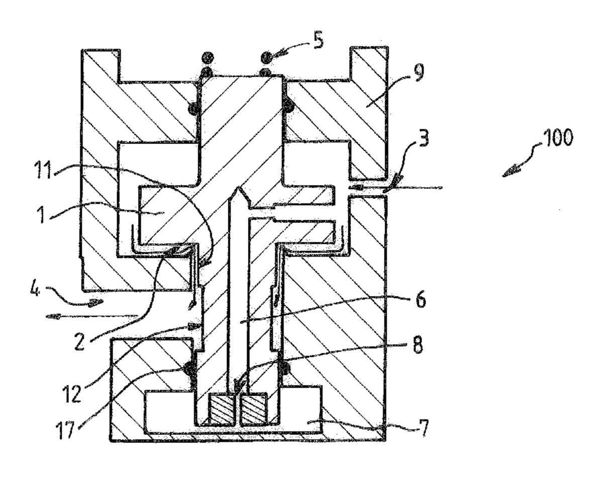
predetermined fit forming a restriction ensuring partial and progressive opening of the passage for the gas between the inlet (3) and the outlet (4).
