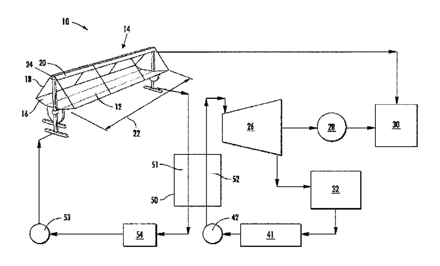
driven by the vapor and electrical power is produced via the rotation of the vapor turbine. Output vapor from the vapor turbine is utilized to drive a thermal conditioning system.
