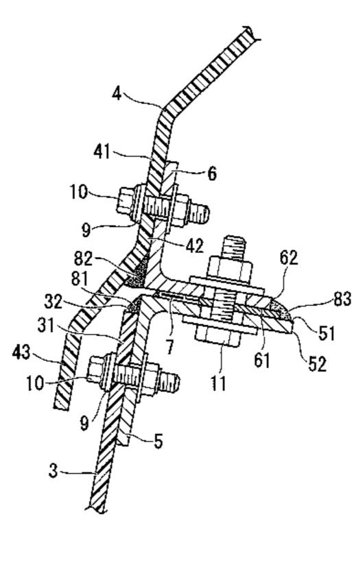
to protrude to the outside of the nacelle cover farther than the lower end portion. A packing is interposed between the upper and lower surfaces.
