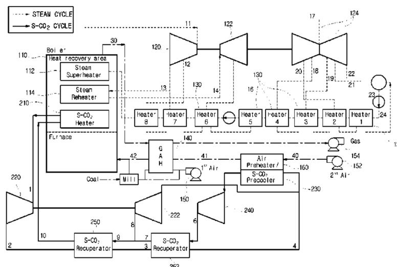
efficiencies of the steam cycle and the supercritical CO<sub>2</sub> cycle by interconnecting the steam cycle and the supercritical CO<sub>2</sub> cycle.
