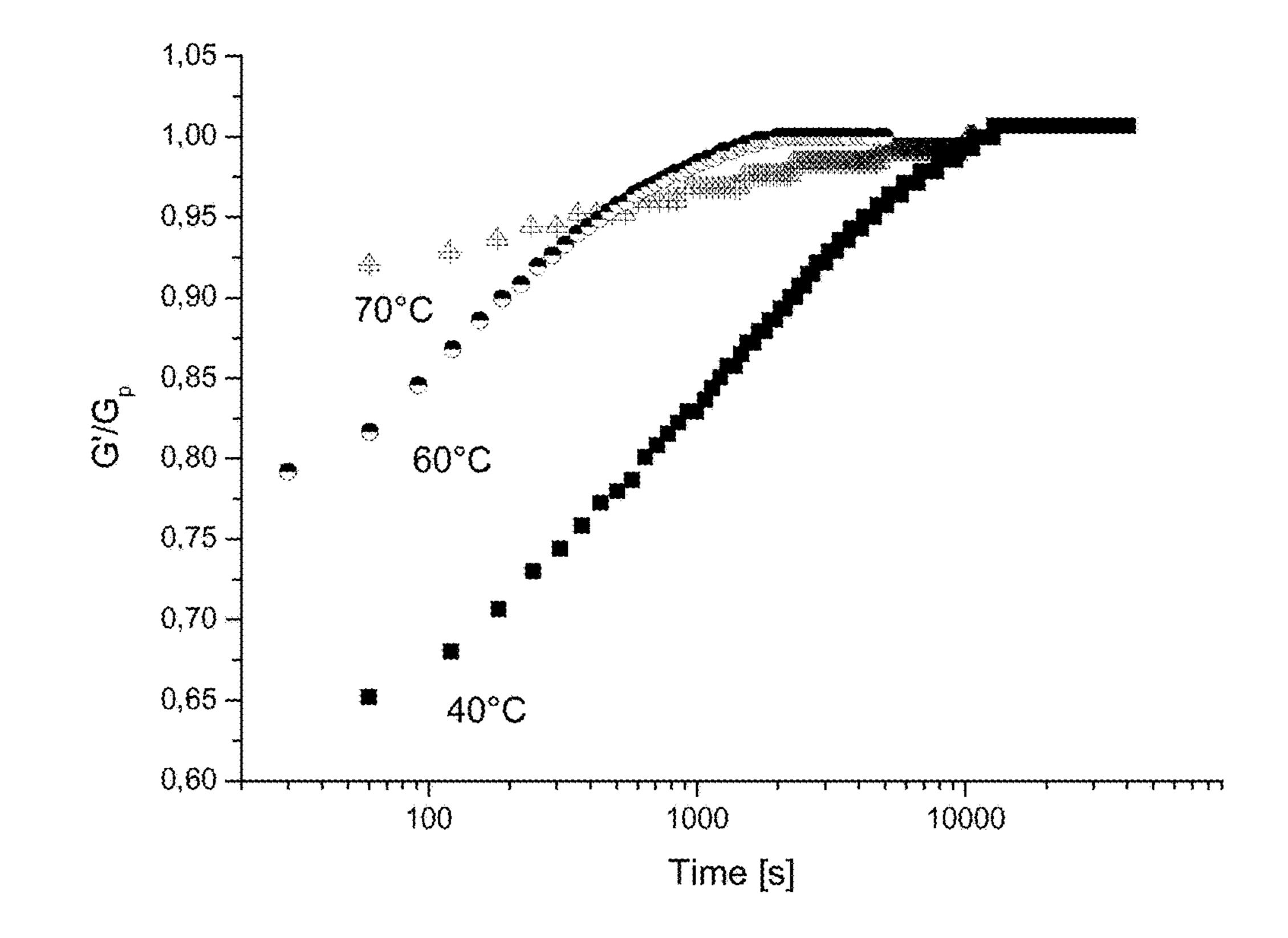
Figure 2: build up of modulus in the disentangled polymer melt with time for IE12 and IE16 and as reference IE17
