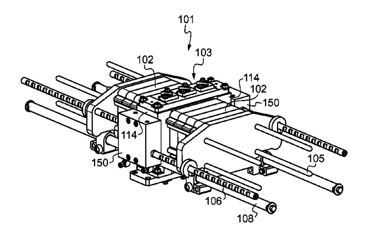
extended position and a retracted position, the body being carried by the manifold, and the member carrying the rod and driving the plate via the rod to a clamped position in which the member is in an intermediate retracted position in which it has moved through a shorter travel than the predetermined travel relative to its extended position.
