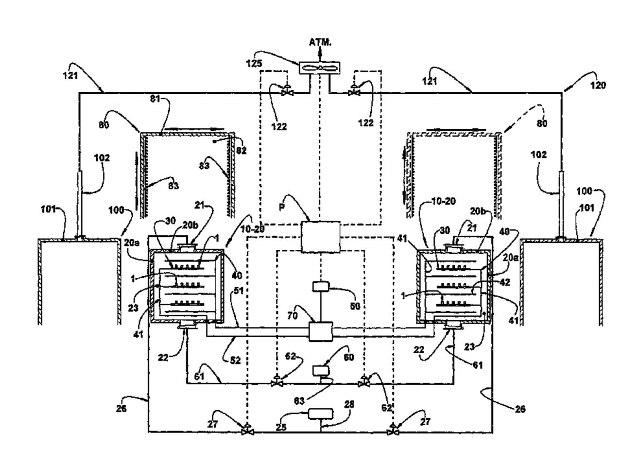
(10), each being selectively and alternately connected to: the same source of ionizable gases (25); the same vacuum source (60); the same electrical energy source (50); and to the same heating device (80), the latter being displaceable between operative positions, in each of which surrounding laterally and superiorly a respective reactor (10), while the latter is in its heating phase (A) and cleaning phase (L) and/or in the surface treatment phase (S) of the metallic pieces (1).
