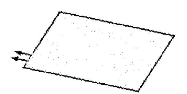
4. Overmold entire piece in urethane or other transparent polymer. Provides double seal & texture.
