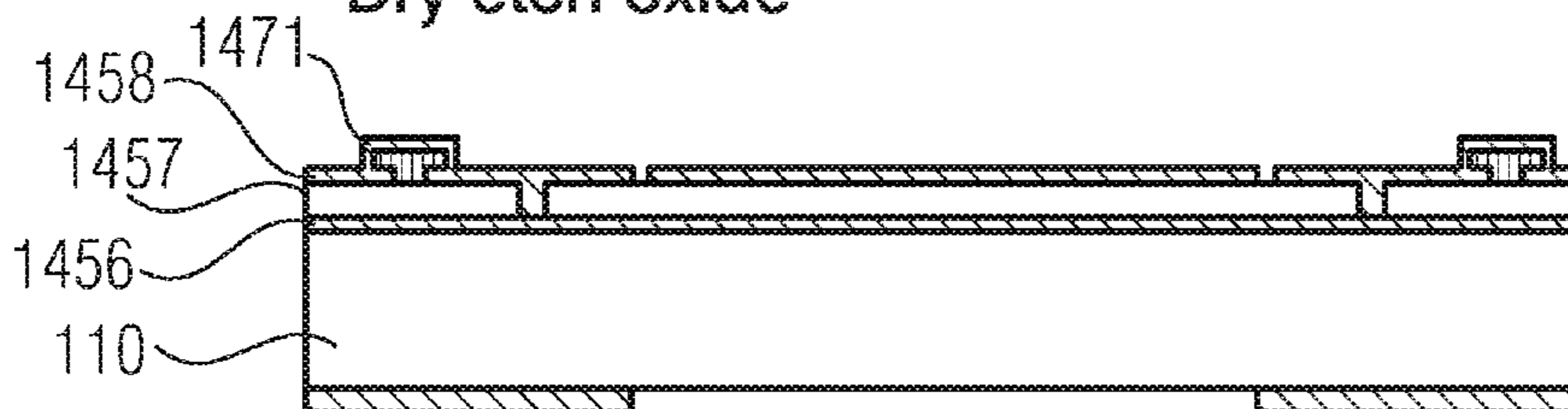
FIG 14F 5. Deposit oxide f Mask: Finger Dry etch oxide
