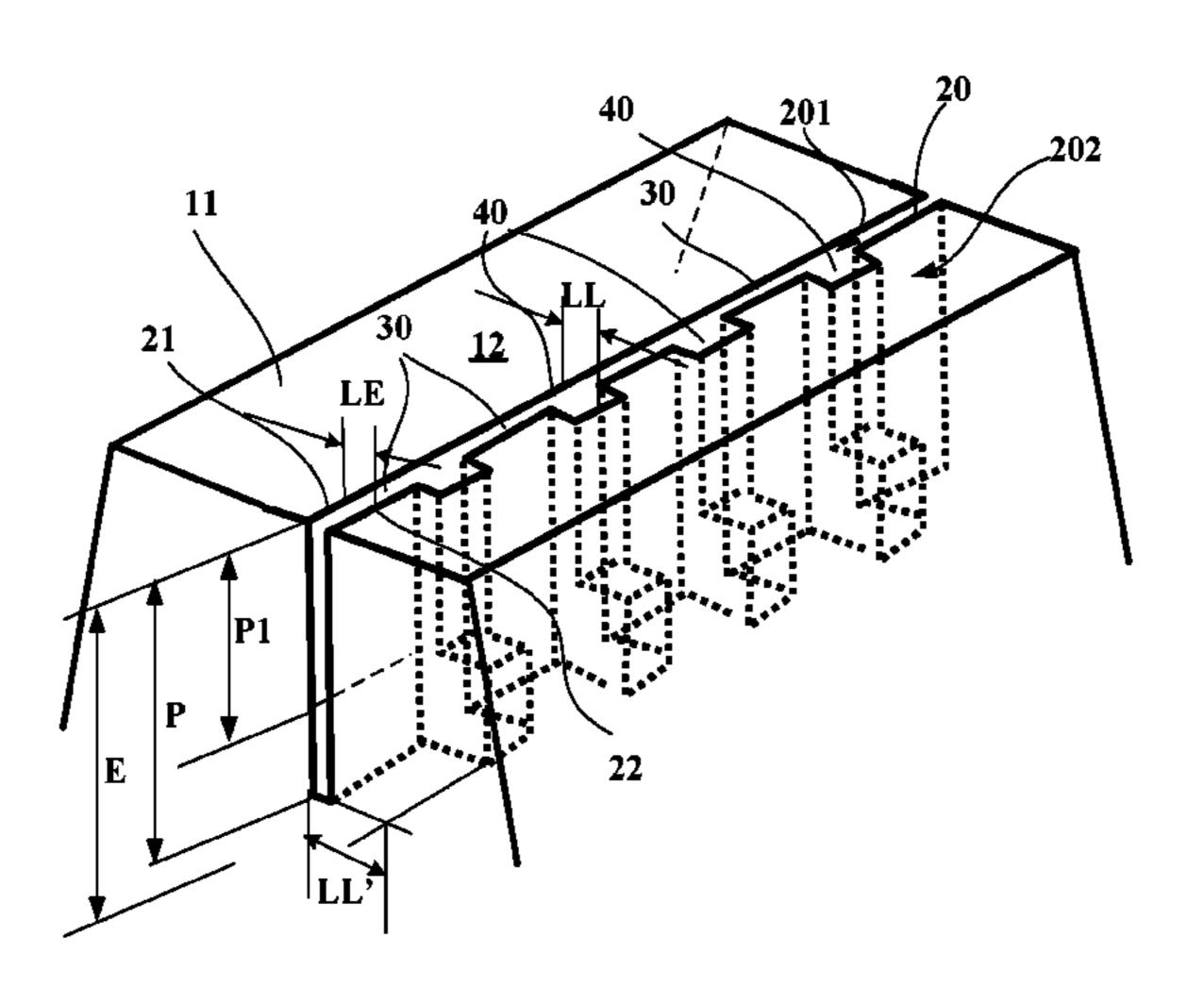
the full depth P of the incision (20), each narrow portion (30) having a volume uniformly distributed over the full depth P of the incision, each wide portion (40) having a volume for the most part between half the depth P of the cut-out and the depth P, this tread being characterized in that the following condition is satisfied:
