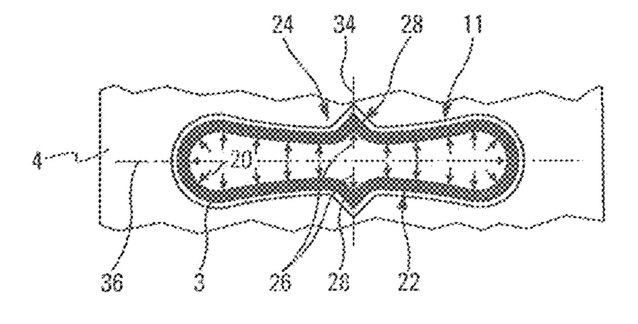
(3), to deform a concave portion (24) of the contour (22) of the tube or tubes (3), in such a way as to correspondingly deform the through holes. A device for implementing the method and an exchanger obtained by the method are also disclosed.
