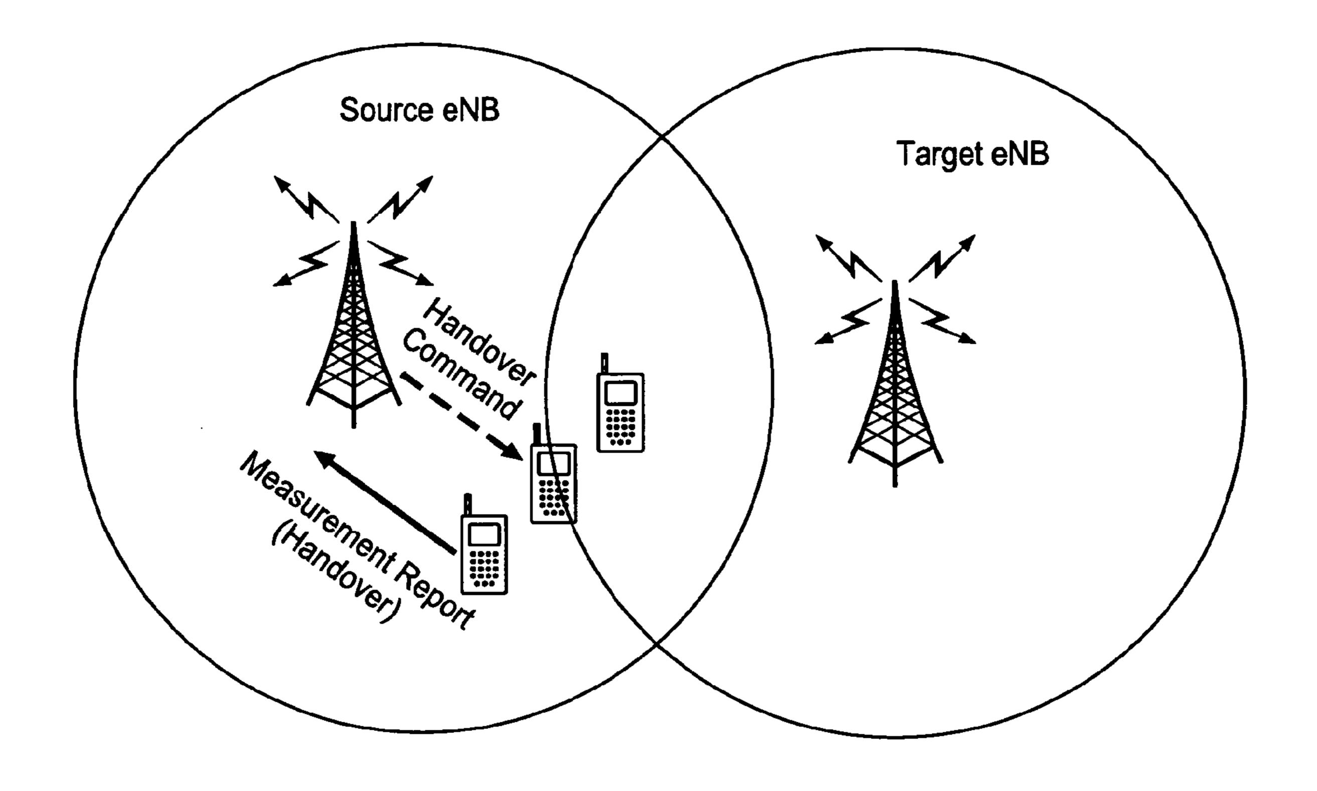
$FIG.\ 3$  Handover Command Failure during LTE Handover
