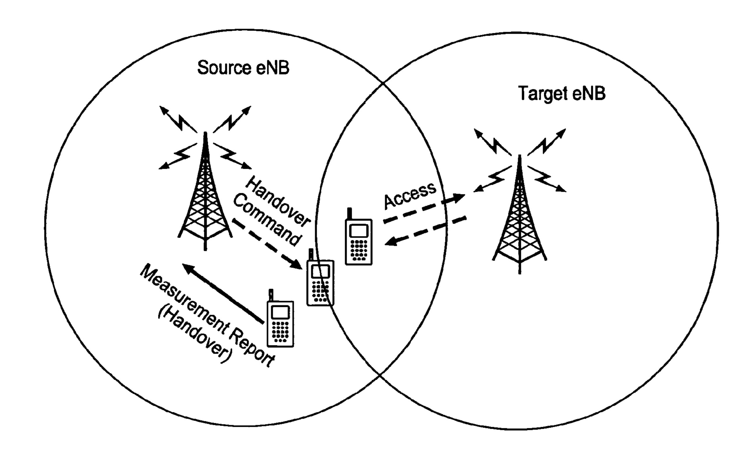
FIG. 4 Access Failure during LTE Handover
