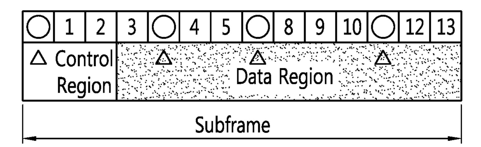
○ Serving cell's CRS△ Interfering cell's CRS
