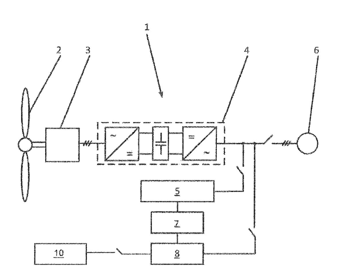
adjustable period of time, and the auxiliary energy unit then draws electrical energy generated by the generator via the converter unit.
