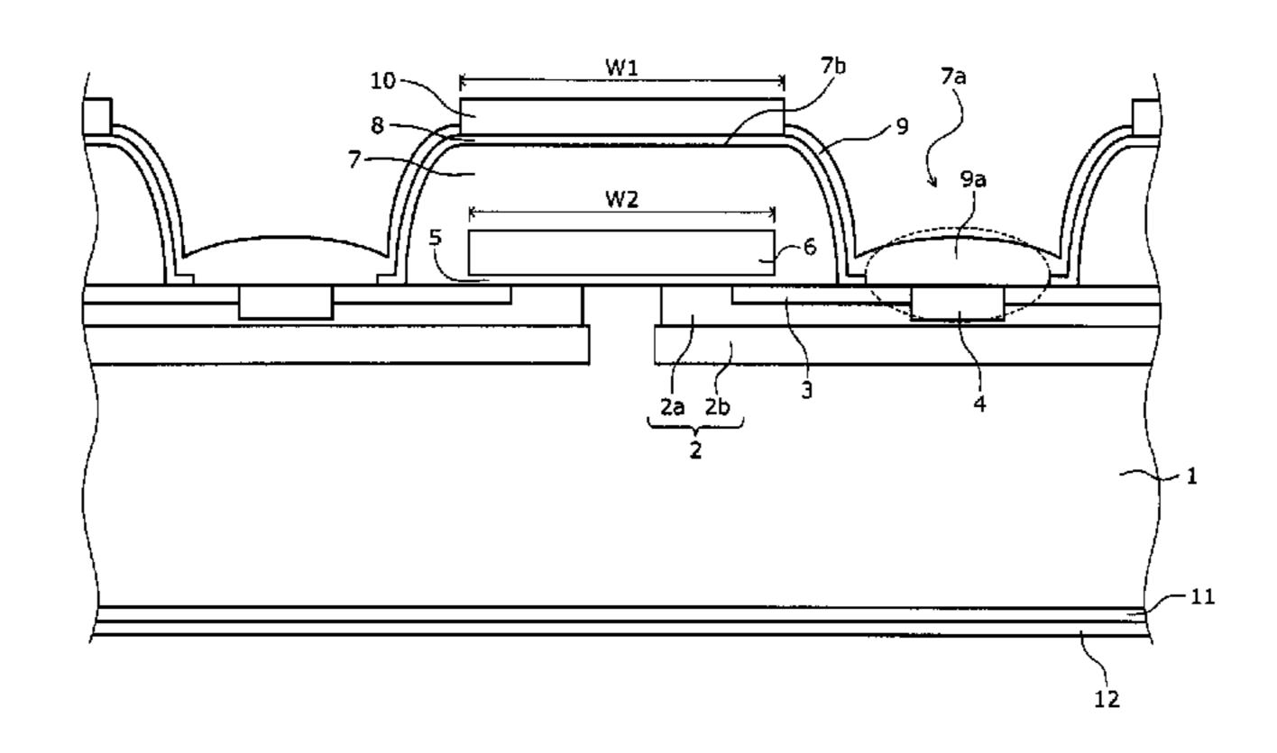
metal film to generate heat and react with the semiconductor substrate and form an ohmic contact there between.
