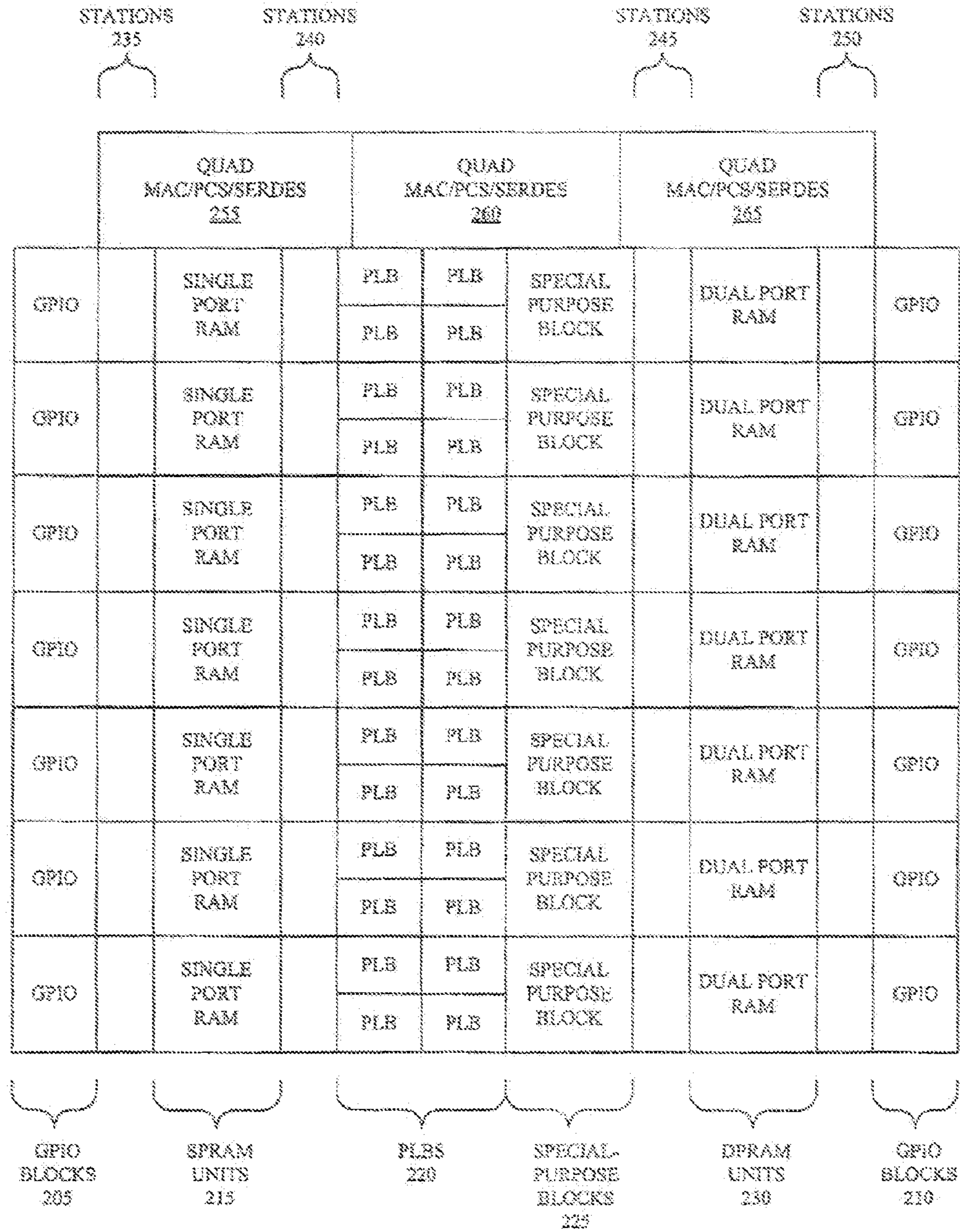
HETEROGENEOUS CONFIGURABLE INTEGRATED CIRCUIT (200)
