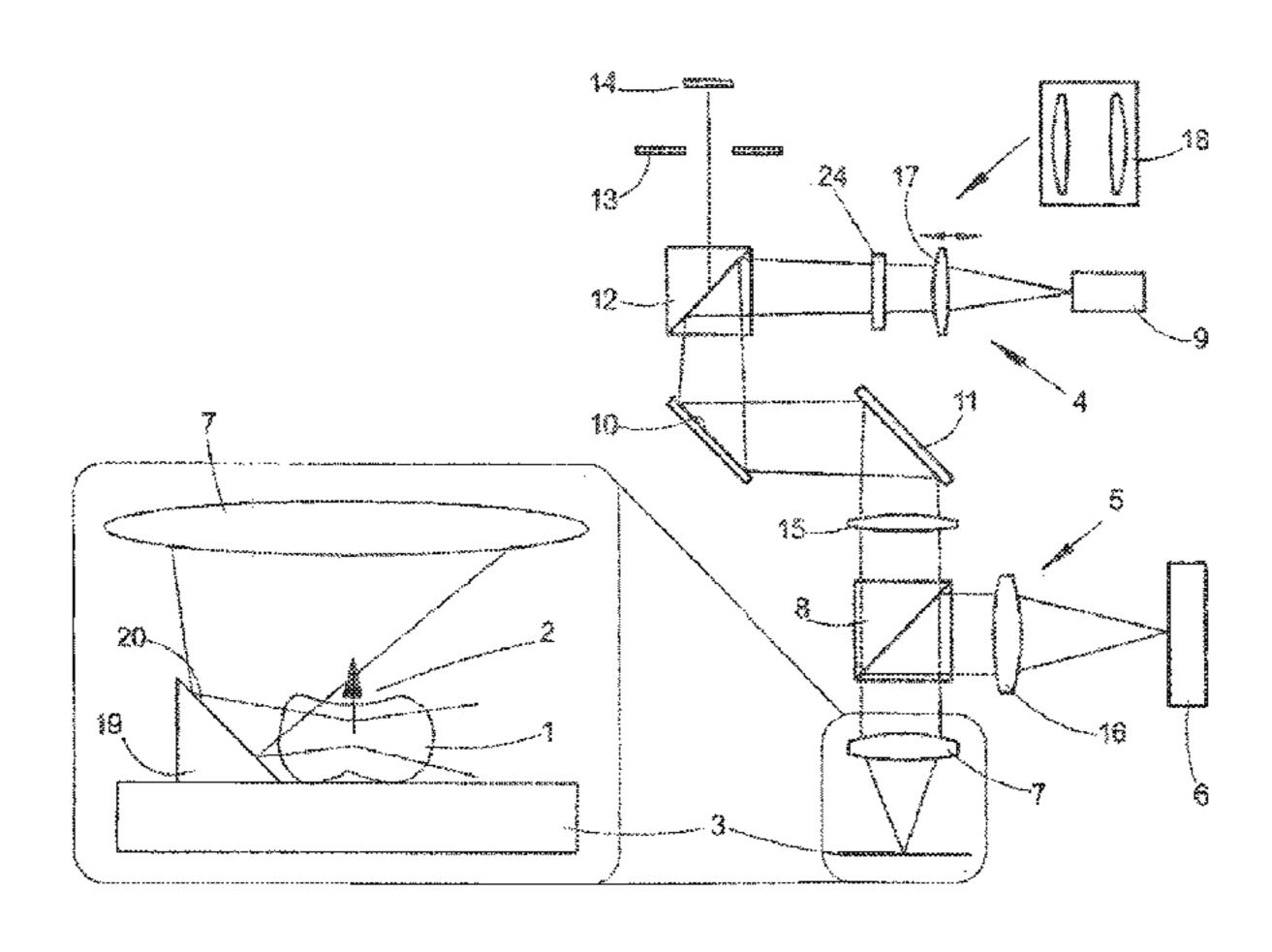
deflecting device arranged on or at the sample carrier, which deflects excitation light from the objective into the plane of the light sheet via an optically active surface.
