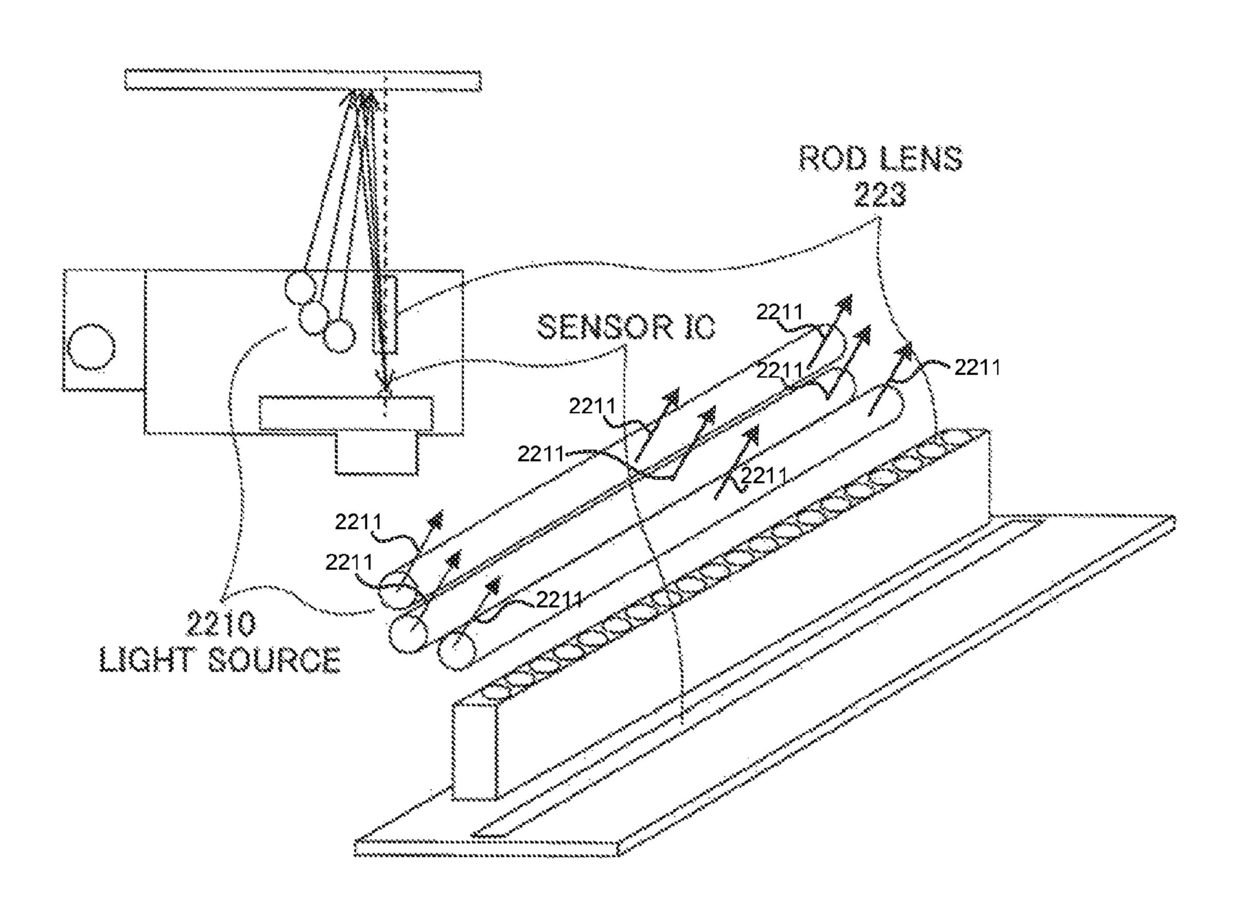
SIDE EDGE DETECTION DEVICE WITH MULTICOLORED LIGHT DETECTION UNIT, IMAGE FORMING APPARATUS PROVIDED WITH THE SIDE EDGE DETECTION DEVICE, SIDE EDGE DETECTION METHOD USING MULTICOLORED LIGHT DETECTION UNIT AND STORAGE MEDIUM THEREOF
