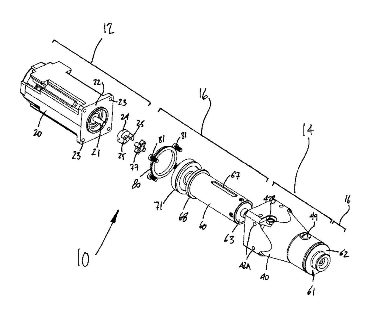
to the sliding tube for moving therewith for converting a rotational motion of the threaded shaft into a translation of the sliding tube.
