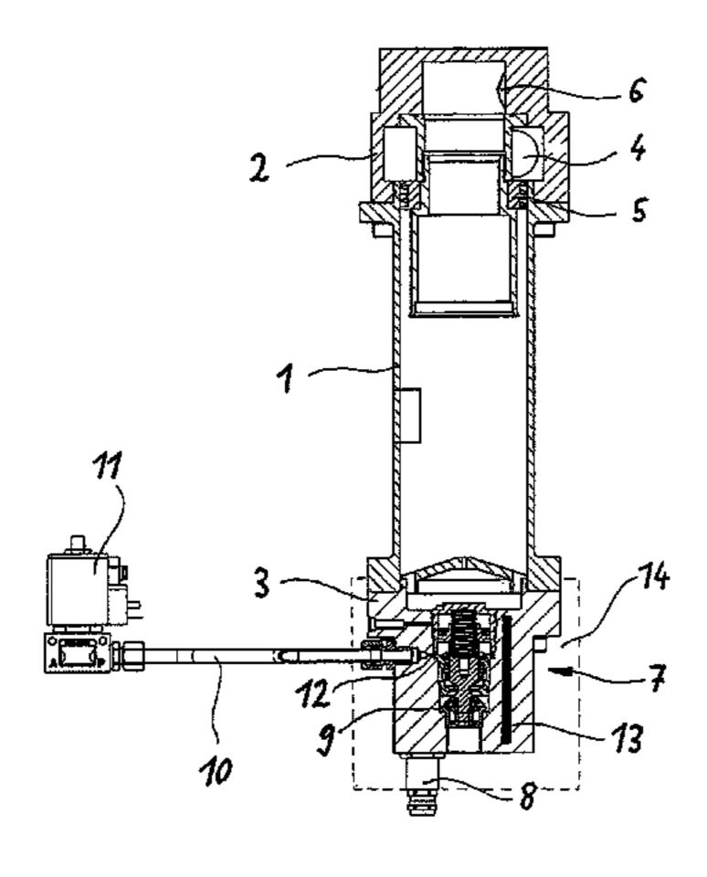
rator housing, into the surrounding environment via a release opening. The valve is pneumatically-piloted seat valve able to be controlled by an electro-pneumatic control valve, and this electro-pneumatic control valve of the drainage valve is arranged outside the separator housing and connected to a pilot connection of the drainage valve via a control pressure-line.
