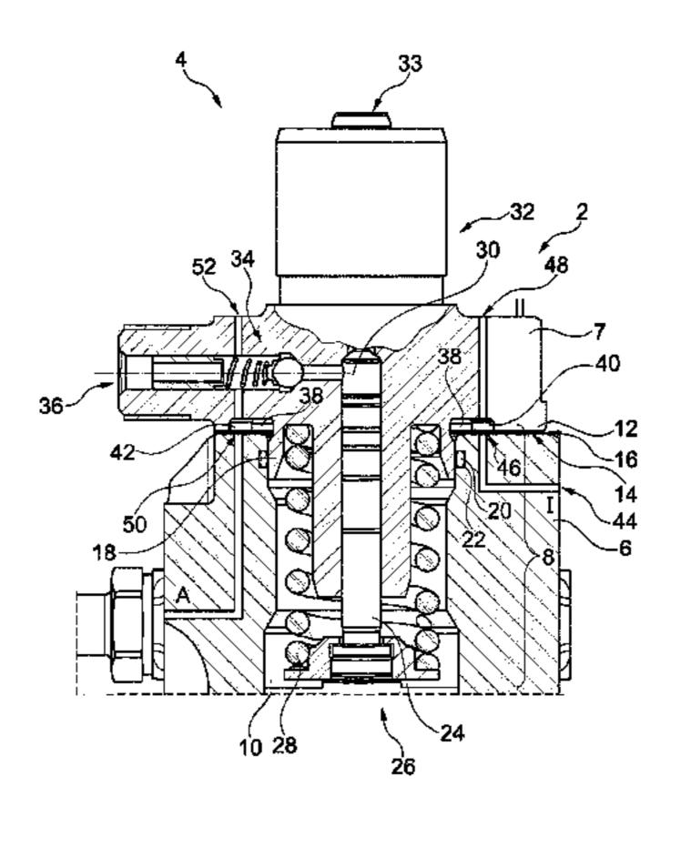
with a separate fluid inlet and a separate fluid outlet. The fluid inlet is connectable to a fluid-discharging line of the internal combustion engine, and the fluid outlet is connectable to a fluid-receiving line of the internal combustion engine.
