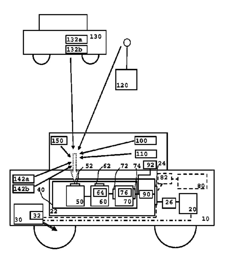
consumption parameter. The consumption parameter characterizes the drive-specific consumption of electrical energy via the electrical assistance traction drive. The method further includes estimating the residual energy by reducing the total amount of energy available by the reserved energy component.
