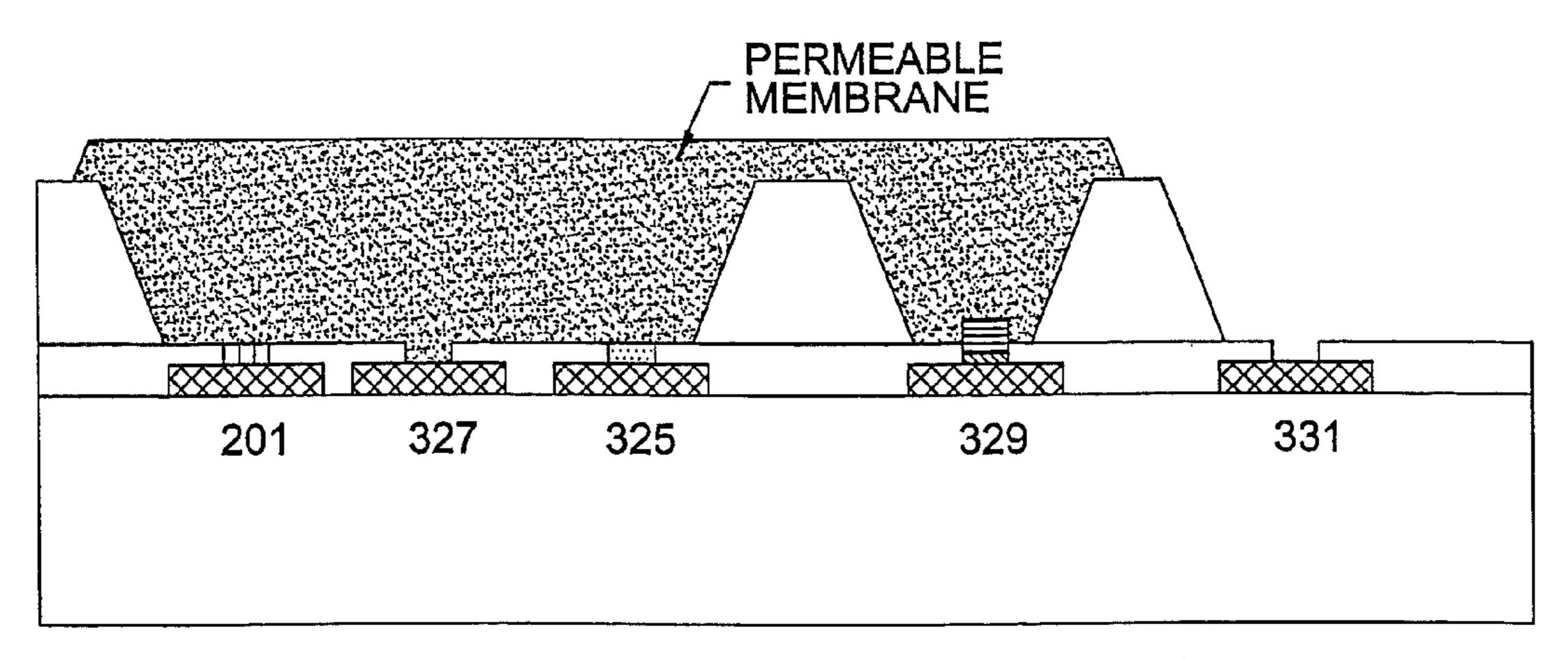
ELECTROPLATING (IrO<sub>2</sub>, Au, AgCI/Ag)
