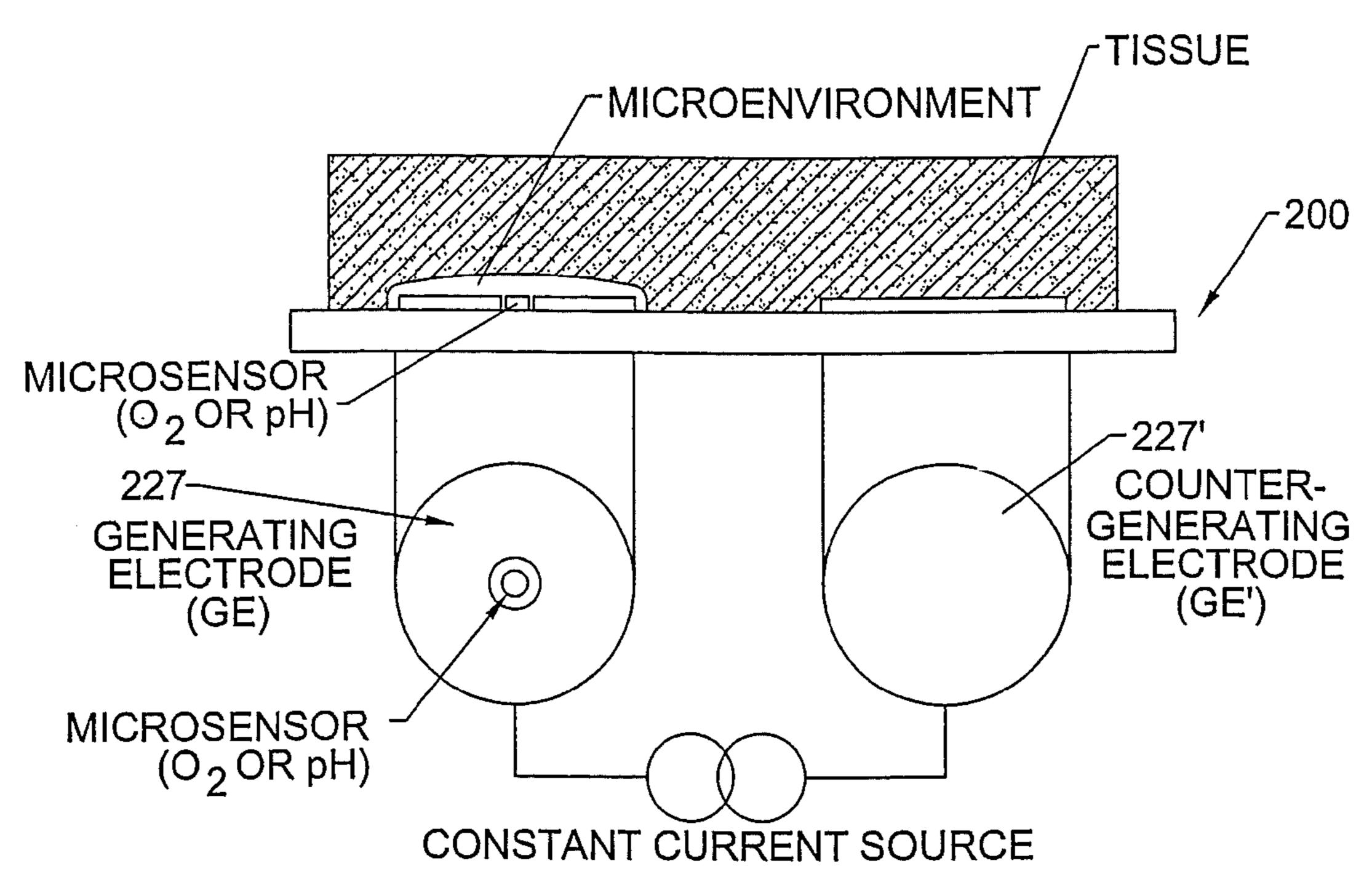
OPERATING PRINCIPLE OF SELF-CALIBRATING, IN SITU, IN VIVO MICROSENSOR. THE MICROENVIRONMENT CONTROLLED BY THE MAGNITUDE AND DIRECTION OF THE GENERATING CURRENT; OXYGEN-SATURATION OR OXYGEN-DEPLETION DEPENDS ON ANODIC OR CATHODIC BEHAVIOR OF GE.
