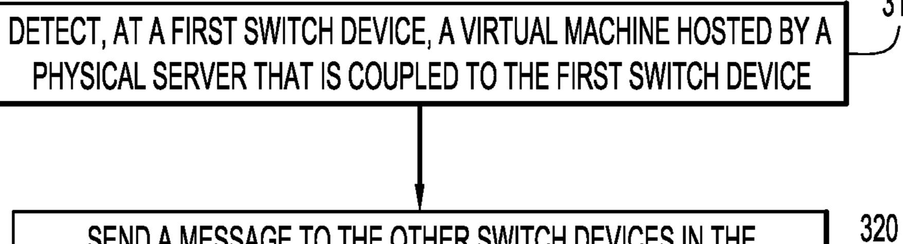
SEND A MESSAGE TO THE OTHER SWITCH DEVICES IN THE NETWORK, WHEREIN THE MESSAGE INDICATEWS THAT THE VIRTUAL MACHINE IS HOSTED BY THE PHYSICAL SERVER THAT IS COUPLED TO THE FIRST SWITCH DEVICE AND WHEN THE FIRST SWITCH DEVICE IS PAIRED WITH A SECOND SWITCH DEVICE AS A VIRTUAL PORT CHANNEL PAIR IN THE NETWORK, THE MESSAGE INCLUDES A SWITCH IDENTIFIER THAT IDENTIFIES THE SECOND SWITCH DEVICE
