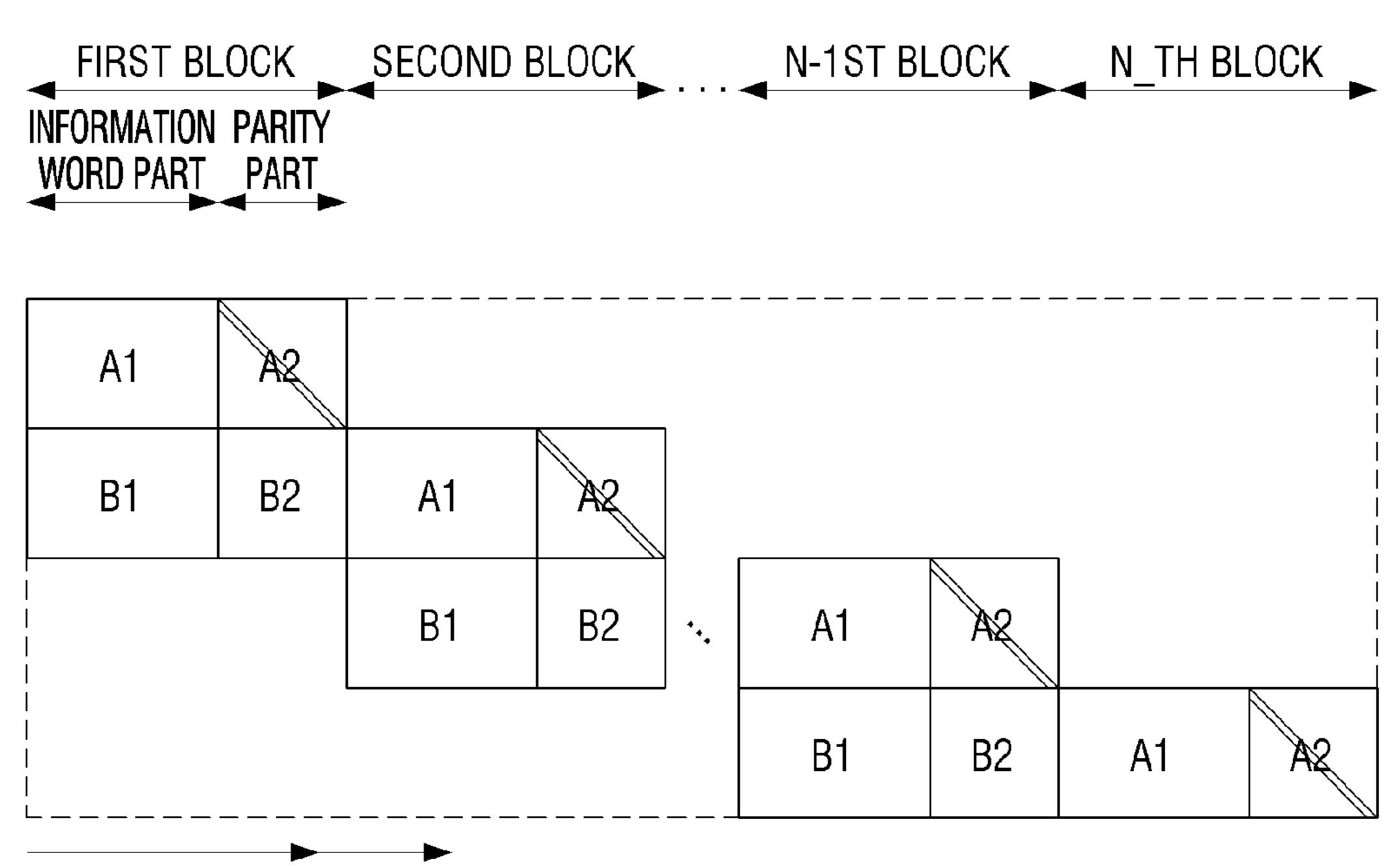
①GENERATE TEMPORARY PARITY ②CALCULATE PARITY BIT THROUGH SEQUENTIAL ACCUMULATION PROCESS
