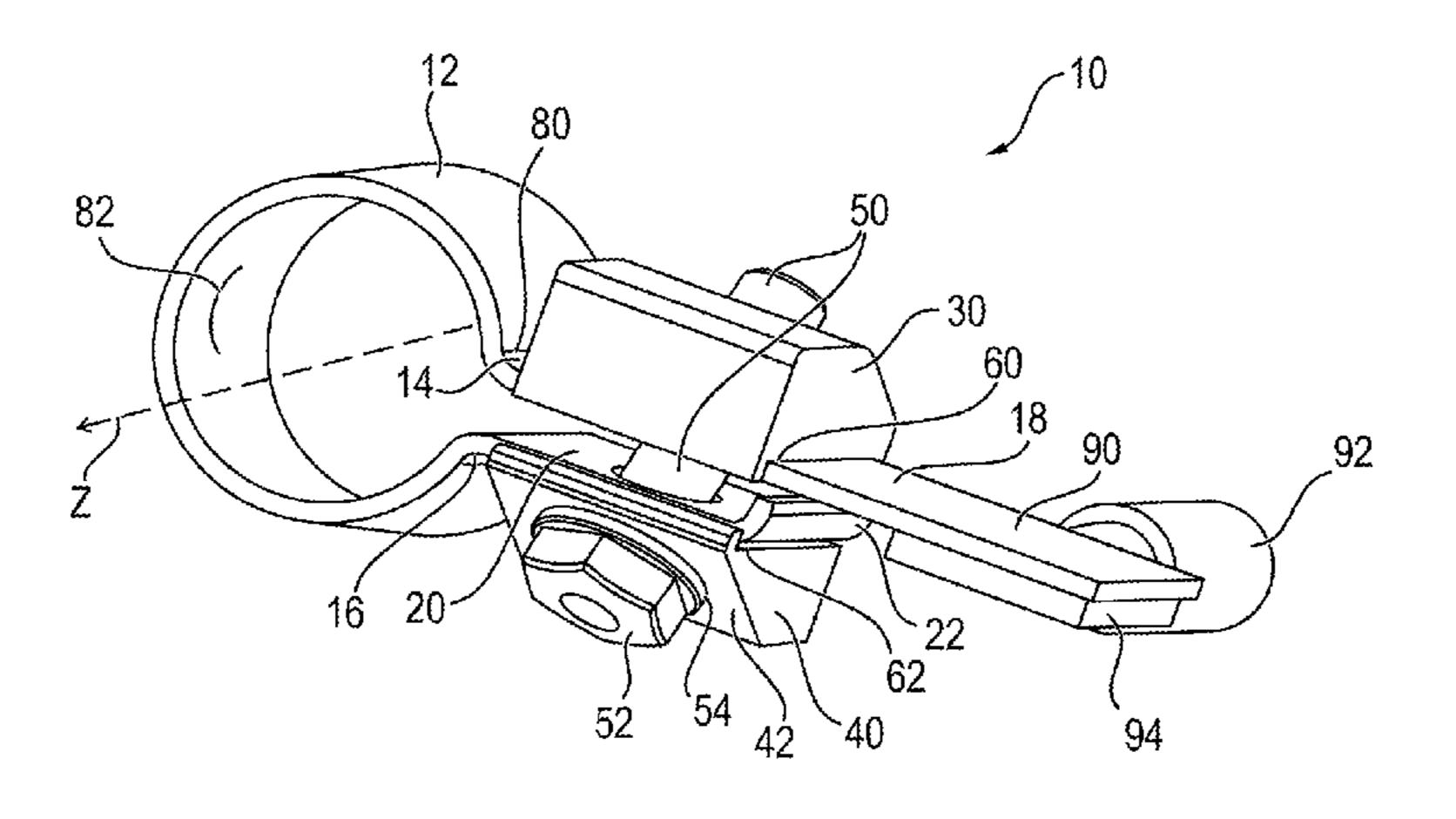
formed in the first clamping piece and a second screw receptacle formed in the second clamping piece, said first and second screw receptacles being aligned with one another along the tensioning direction.
