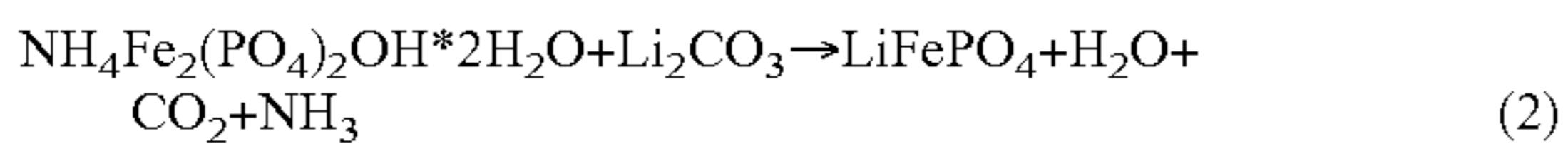
The spheniscidite may be obtained by reacting an iron source, an ammonium source, and an oxidant. The spheniscidite obtained has a single-phase and a high purity. The spheniscidite may have a surface area in a range of  $20 \text{ m}^2/\text{g}$  to  $25 \text{ m}^2/\text{g}$ . For example, in some embodiments, the plate-shaped single-phase spheniscidite precursor may have a surface area of about  $23 \text{ m}^2/\text{g}$ .
