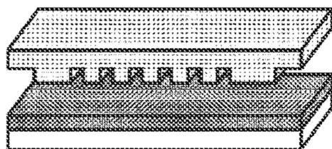
2. Put a metal cast on a polymer
