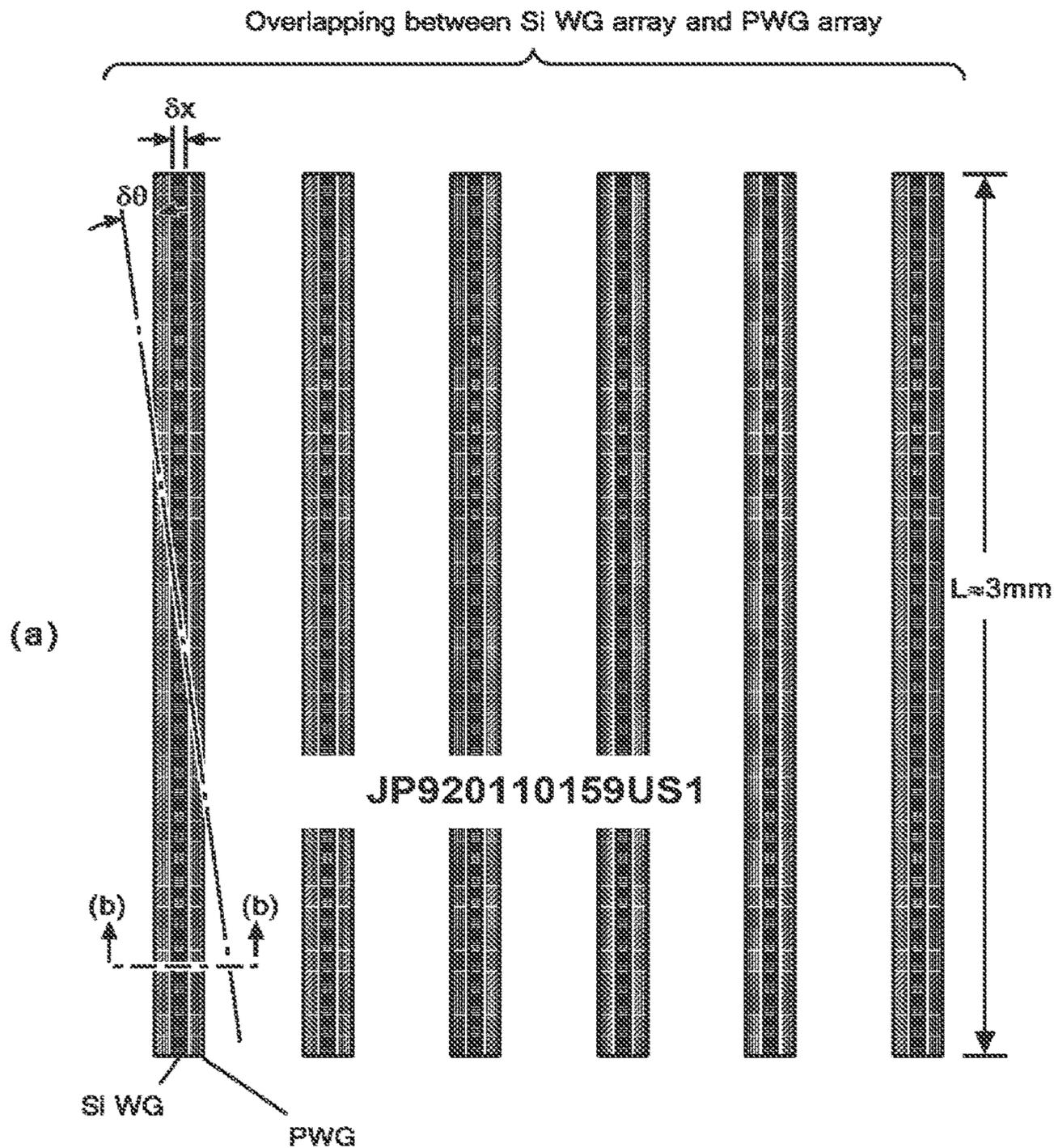
High precision overlapping is required for adiabatic coupling
