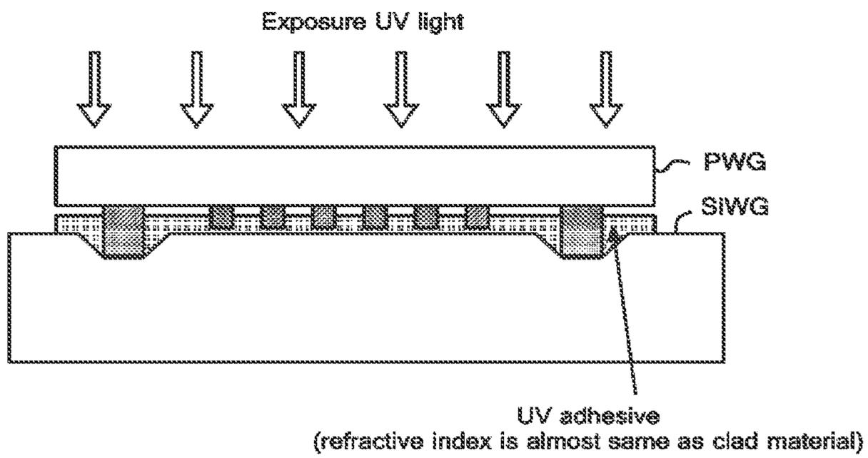
Fix using UV adhesive between Si wafer and PWG
