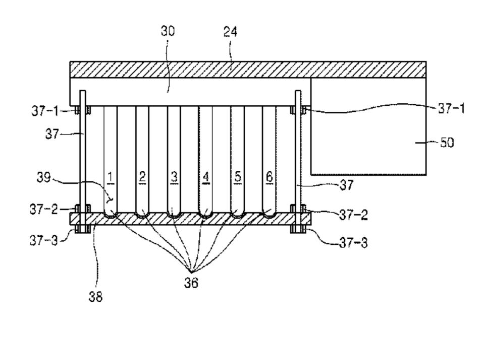
collected through the funnel are fixedly attached, is formed under the fixing plate. The container fixing holder includes a circular holder for fixing the plurality of time-series sediment trapping containers fixedly attached to the rotation plate without shaking.
