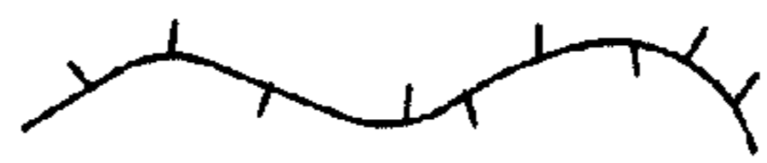
Linear-low-density polyethylene (LLDPE) (High degree of short-chain branching)
