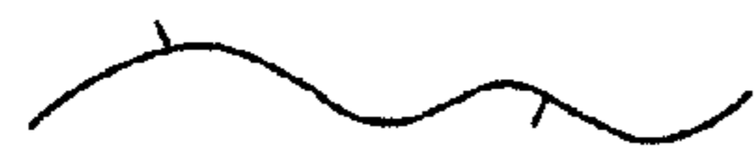
High-density polyethylene (HDPE) (Low degree of short-chain branching)
