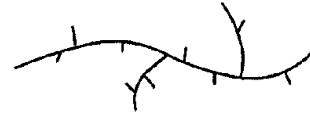
Low-density polyethylene (LDPE) (High degree of short-chain branching + long-chain branching)
