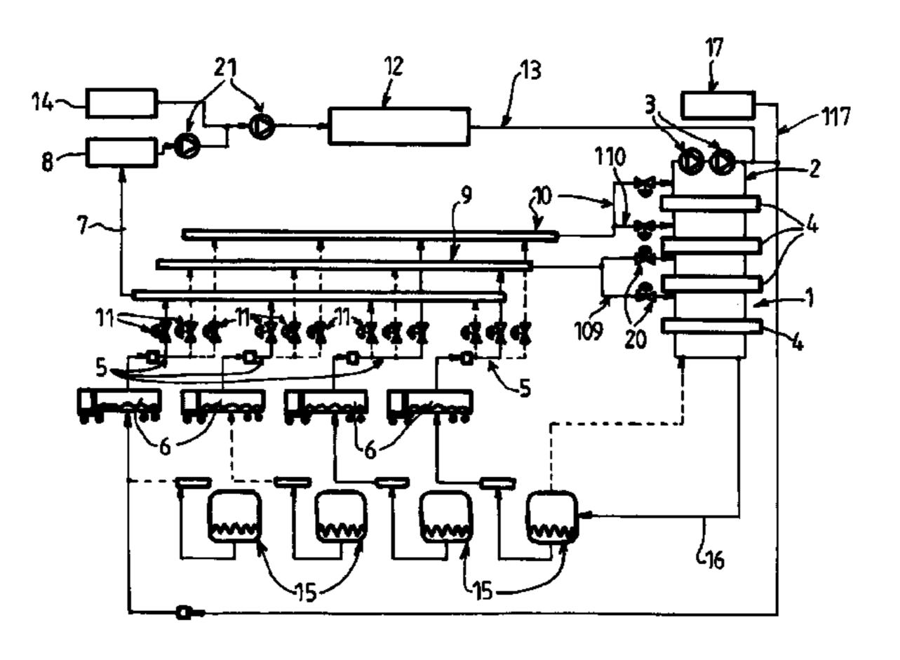
the recovery lines and a downstream end connected to the working circuit, the upstream ends of the second and third collection lines being connected at separate determined positions of the working circuit, that respectively correspond to separate temperature levels of the working fluid in the working circuit.
